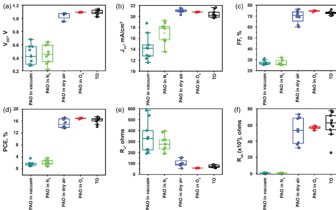
Fig. 4 Statistical distribution diagram of the photovoltaic parameters of the PSCs prepared with TO and PAO Spiro-OMeTAD in different conditions. (a)  $V_{OC}$ , (b)  $J_{SC}$ , (c) fill factor, FF, (d) PCE, (e)  $R_s$ , and (f)  $R_{sh}$ .
