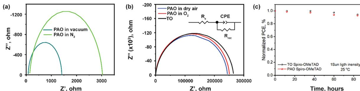
**Fig. 6** (a) Nyquist plot for the devices with PAO Spiro-OMeTAD in vacuum and N<sub>2</sub>, and (b) Nyquist plot for the devices with TO and PAO Spiro-OMeTAD in O<sub>2</sub> and dry air. (c) Light soaking stability test for the TO and PAO Spiro-OMeTAD based perovskite solar cells with a carbon electrode.
