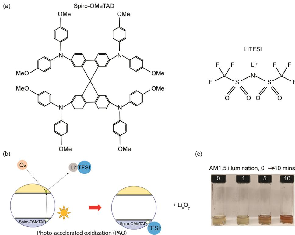
Fig. 1 (a) Molecular structures of Spiro-OMeTAD and LiTFSI, (b) schematic of the proposed PAO mechanism of Spiro-OMeTAD, and (c) optical pictures of the Spiro-OMeTAD solution illuminated under 1 sun sunlight after 0, 1, 5, and 10 minutes of PAO treatment in  $O_2$ .
