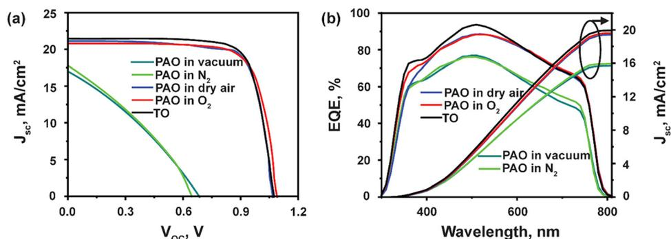
Fig. 3 (a) *J-V* characteristics and, (b) EQE spectra of PSCs using TO and PAO Spiro-OMeTAD in different conditions.
