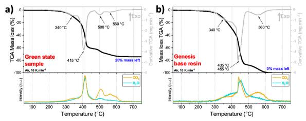
Fig. 3 (a) TG (top) and MS (bottom) analysis of the composite resin containing  $LiCoO_2$  and carbon black C45 materials in the green state (before thermal post-processing). (b) TG (top) and MS (bottom) analysis of the Genesis base resin.
