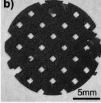
(a) Picture of the actual 100% infill printed disc from the primary resin and (b) of the 90% infill. The diameter corresponds to the size of a coin cell battery used for electrochemical characterization.
