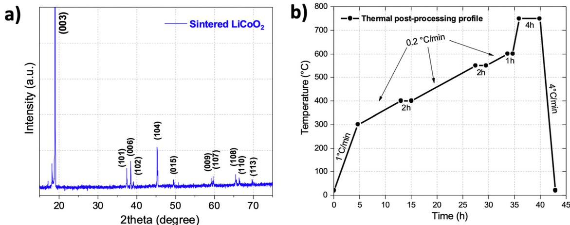
Fig. 4 (a) XRD diffractogram obtained from the residues left from thermal post-processing. The reflections of  $\text{LiCoO}_2$  are indicated in parentheses. (b) Thermal post-processing profile including debinding and sintering steps.
