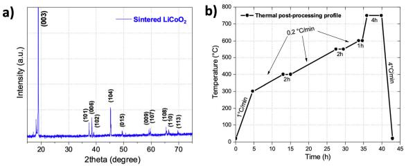
Fig. 4 (a) XRD diffractogram obtained from the residues left from thermal post-processing. The reflections of LiCoO<sub>2</sub> are indicated in parentheses. (b) Thermal post-processing profile including debinding and sintering steps.
