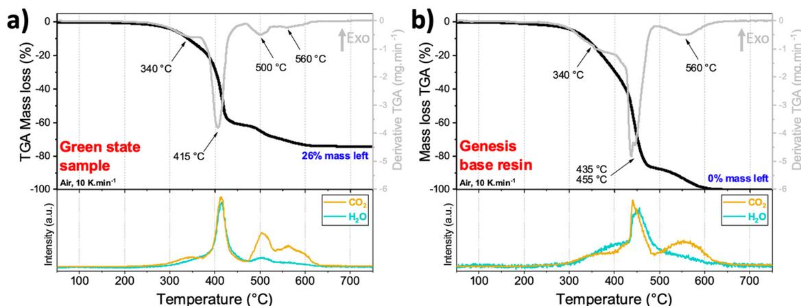
Fig. 3 (a) TG (top) and MS (bottom) analysis of the composite resin containing  $\text{LiCoO}_2$  and carbon black C45 materials in the green state (before thermal post-processing). (b) TG (top) and MS (bottom) analysis of the Genesis base resin.
