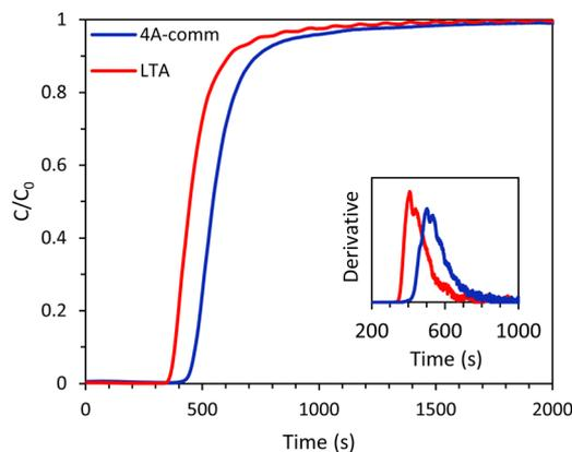
Fig. 4 CO<sub>2</sub> breakthrough curves of the LTA and 4A-comm beads. In the inset, the derivative of the breakthrough curves is displayed. Feed: 40 vol% CO<sub>2</sub> and 60 vol% CH<sub>4</sub> (mimicking biogas).
