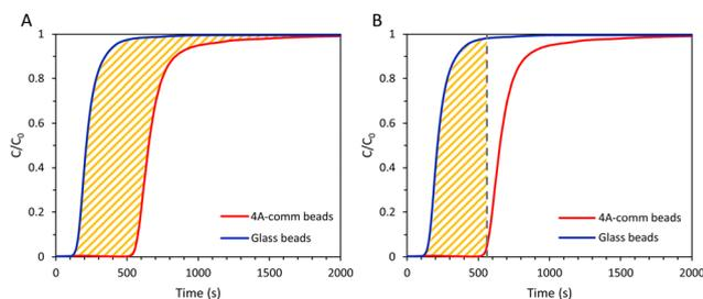
Fig. 2 (A) Area between the breakthrough curve of the glass beads and that of the adsorbent (yellow) for CO<sub>2</sub> adsorption capacity at full utilization; (B) area between the vertical line from the breakthrough time,  $t_{\text{b}}$ , and the breakthrough curve of the glass beads (yellow) for CO<sub>2</sub> adsorption capacity at breakthrough.
