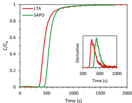
Fig. 8 CO<sub>2</sub> breakthrough curves of the LTA and SAPO-34 beads. The inset displays the derivative of the breakthrough curves. Feed: 40 vol% CO<sub>2</sub> and 60 vol% CH<sub>4</sub> (mimicking biogas).
