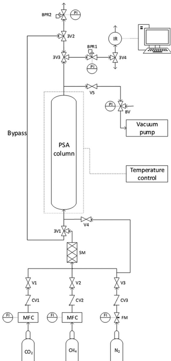
**Fig. 1** Schematic overview of the experimental setup for conducting VPSA breakthrough experiments. V = valve; 3V = three-way valve; BV = bleeding valve (regulating the reduced pressure); CV = check valve (preventing back-flow); FI = flow indicator; FM = variable area flowmeter; MFC = mass flow controller; SM = static mixer; BPR = back pressure regulator; PI = pressure indicator; IR = infrared CO<sub>2</sub> sensor.
