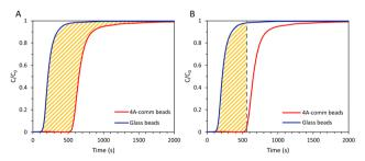
Fig. 2 (A) Area between the breakthrough curve of the glass beads and that of the adsorbent (yellow) for  $CO_2$  adsorption capacity at full utilization; (B) area between the vertical line from the breakthrough time,  $t_{\rm b}$ , and the breakthrough curve of the glass beads (yellow) for  $CO_2$  adsorption capacity at breakthrough.
