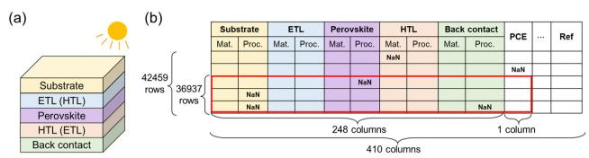
Fig. 1 The structures of perovskite solar cell and the Perovskite Database. (a) Typical structure of nip-type cell, and the bracket represents the pin-type structure. (b) The size and information of the Perovskite Database. The curated dataset used in this work is shown by red boxed line.
