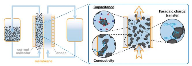
Fig. 1 Suspension based electrochemical flow system (left) and charge transfer mechanisms inside the flowing suspension electrode (right). Charge transfer takes place through electric double layer charging (capacitive charge storage), electric conductivity via particle networks, and faradaic charge transfer, in this example CO2 reduction to CO.
