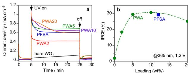
Fig. 4 Photocurrent response of the  $\text{WO}_3$  photoanodes in a continuous flow of humidified argon (RH < 90%) under UV irradiation (365 nm, 7.0  $\text{mW cm}^{-2}$ , area 2  $\text{cm}^2$ ). (a) Photocurrent response of  $\text{WO}_3$  photoanodes coated with PFSA and PWA with different loading amount (wt%) at 1.2 V vs. Pt-CB cathode. (b) Incident photon-to-current conversion efficiency (IPCE) at 1.2 V.
