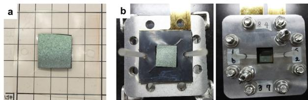
Fig. 3 (a) Membrane electrode assembly composed of the  $\text{WO}_3$  photoanode, N117, and the Pt-CB electrocatalyst. (b) Planar-type stainless steel cell for gas-fed PEC reaction with an irradiation window of 2  $\text{cm}^2$ .
