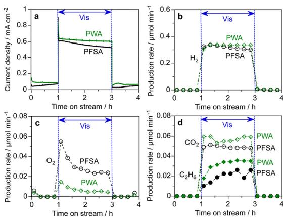
**Fig. 8** PEM-PEC methane conversion reactions using the PWA/WO<sub>3</sub> and PFSA/WO<sub>3</sub> photoanodes at 1.2 V (vs. Pt–CB) under visible light irradiation (453 nm, 22 mW cm<sup>-2</sup>, and area 2 cm<sup>2</sup>): (a) photocurrent response, (b) H<sub>2</sub> production rate at the cathode, (c) O<sub>2</sub> production rate at the photoanode and (d) production rate of CO<sub>2</sub> and C<sub>2</sub>H<sub>6</sub> at the photoanode.
