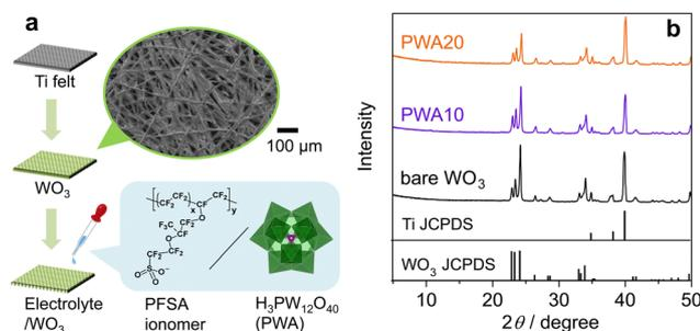
Fig. 1 (a) Preparation of porous  $\text{WO}_3$  photoanode and surface electrolyte coating. (b) XRD patterns of PWA/ $\text{WO}_3$  photoanodes and the standard lines of  $\text{WO}_3$  (JCPDS No. 01-072-0677) and Ti (JCPDS No. 00-044-1294).
