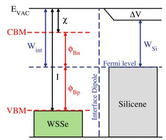
Fig. 3 Schematics of the silicene/Janus heterojunction.  $E_{vac}$  is the vacuum level and the horizontal blue dashed lines are the Fermi level  $E_f$ of the interface. The  $W_{Si}$  ( $W_{int}$ ) is the work function of the silicene (interfaces),  $\chi$  (/) is the electron affinity (ionization potential) of the WSSe and the  $\phi_{\rm Bn}$  ( $\phi_{\rm Bp}$ ) are the n-type (p-type) Schottky barrier height.
