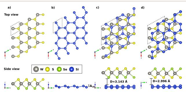
Fig. 1 The fully relaxed geometries are shown, where (a) represents the WSSe Janus monolayer, (b) the silicene monolayer, and (c) and (d) the WSSe/Si (Se atoms are the shortest distance from Si atoms) and WSeS/Si (S atoms are the shortest distance from Si atoms) heterostructures, respectively
