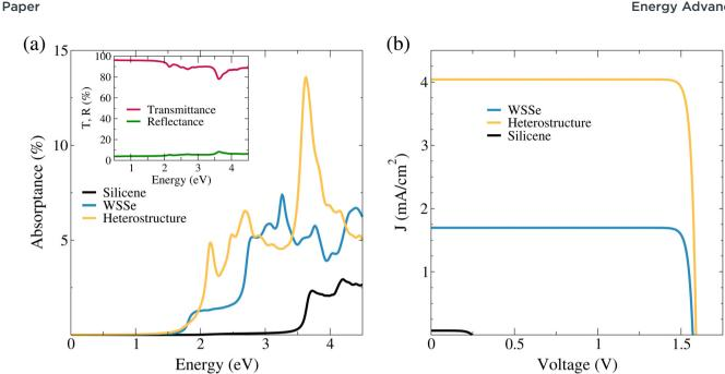
Fig. 4 (a) Optical absorptance of monolayer WSSe (blue), silicene (black), and the WSSe/Si interface (yellow). (b) Current density as a function of voltage for the three studied systems. The inset shows the transmittance (red) and reflectance (green) of the WSSe/Si interface.
