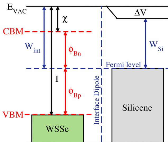
**Fig. 3** Schematics of the silicene/Janus heterojunction.  $E_{\text{vac}}$  is the vacuum level and the horizontal blue dashed lines are the Fermi level  $E_F$  of the interface. The  $W_{\text{Si}}$  ( $W_{\text{int}}$ ) is the work function of the silicene (interfaces),  $\chi$  ( $I$ ) is the electron affinity (ionization potential) of the WSSe and the  $\phi_{\text{Bn}}$  ( $\phi_{\text{Bp}}$ ) are the n-type (p-type) Schottky barrier height.
