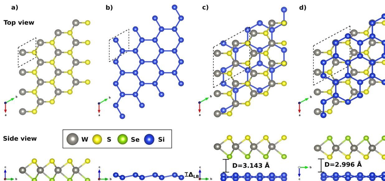
**Fig. 1** The fully relaxed geometries are shown, where (a) represents the WSSe Janus monolayer, (b) the silicene monolayer, and (c) and (d) the WSSe/Si (Se atoms are the shortest distance from Si atoms) and WSeS/Si (S atoms are the shortest distance from Si atoms) heterostructures, respectively.
