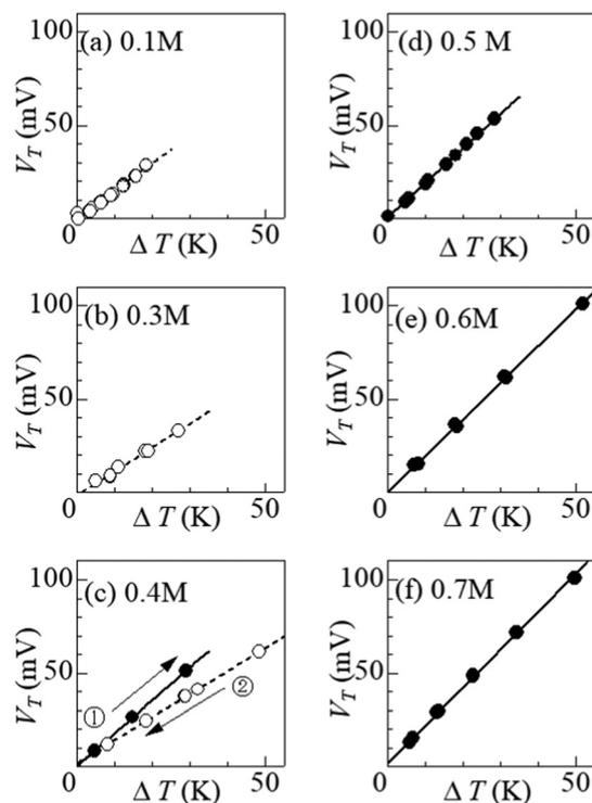
Fig. 4 Thermoelectromotive force  $V_{\text{T}}$  against temperature difference  $\Delta T$  in DMF containing  $m$  M  $\text{Fe}(\text{ClO}_4)_2$  and  $m$  M  $\text{Fe}(\text{ClO}_4)_3$ : (a)  $m = 0.1$  M, (b) 0.3 M, (c) 0.4 M, (d) 0.5 M, (e) 0.6 M, and (f) 0.7 M. Closed and open circles correspond to electrolytes with and without precipitates, respectively. Straight lines are the results of least-squares fitting. Numbers in (c) indicate the order of measurements.
