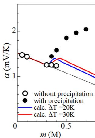
Fig. 5 Electrochemical Seebeck coefficient ( $\alpha$ ) against solute concentration  $m$ . Closed and open circles correspond to the observed data with and without precipitates, respectively. The thin straight line is the result of least-squares fitting of the data below 0.3 M without precipitation. The thick blue (red) curve is the calculation based on the concentration gradient model at  $\Delta T = 20 \text{ K}$  (30 K).
