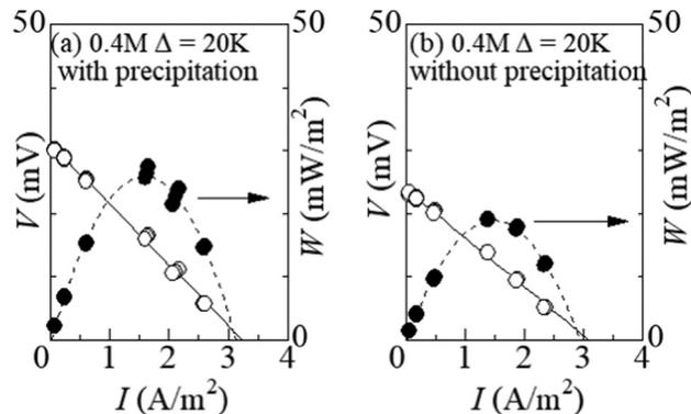
Fig. 6 Output voltage  $V$  and power density  $W$  against current density  $I$  in the LTEs at  $\Delta T = 20 \text{ K}$  at 0.4 M: (a) with and (b) without precipitation. Solid straight lines are the results of least-squares fitting. Broken curves are the result of least-squares fitting with a quadratic function.
