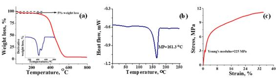
Fig. 3 Thermal and mechanical stability evaluation of the T-CEM. (a) TGA spectra; inset figure: first order derivative graph. (b) Differential scanning calorimetry (DSC) spectra and (c) universal testing machine (UTM) analysis of the T-CEM.
