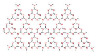
Fig. 2 Schematic illustration of g-C<sub>3</sub>N<sub>4</sub> containing tris-s-triazine units.
