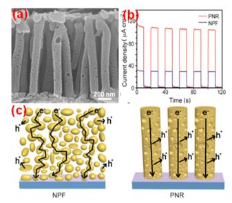
(a) SEM images, (b) transient photocurrent density curves and (c) schematic diagrams showing the transport pathway of electrons in the NPF and PNR of g-C<sub>3</sub>N<sub>4</sub>. Reprinted from ref. 154 with permission.
