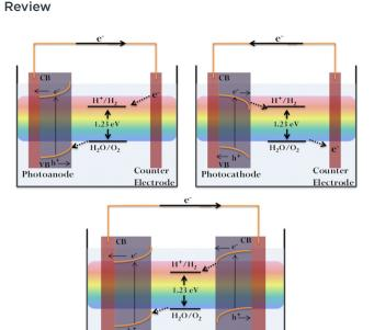
Fig. 1 Schematic representation of PEC water-splitting cells with single and coupled photosystems
