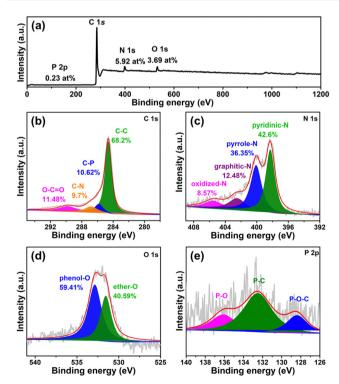
Fig. 2 (a) XPS survey spectrum of 3D-NPOC. High-resolution XPS spectra of (b) C 1s, (c) N 1s, (d) O 1s, and (e) P 2p for 3D-NPOC.
