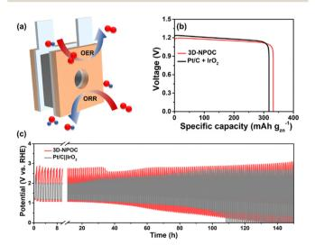
Fig. 6 (a) The schematic diagram of a homemade zinc-air battery. (b) Specific capacities, and (c) battery cycling test of 3D-NPOC and Pt/C + IrO2-based batteries
