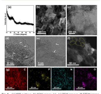
Fig. 1 (a) XRD pattern, (b) SEM image, (c)-(e) TEM images, (f) STEM image, and (g) corresponding elemental mappings of 3D-NPOC.
