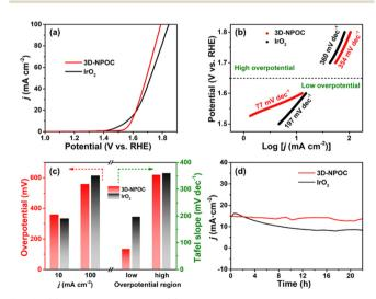
Fig. 4 (a) Polarization curves; (b) Tafel slopes derived from the corresponding polarization curves; (c) histogram of overpotentials at 10 and 100 mA cm $^{-2}$ , and Tafel slopes at different overpotential regions; and (d) durability evaluation at a constant potential of 3D-NPOC and IrO $_2$  for alkaline OER in 1.0 M KOH.
