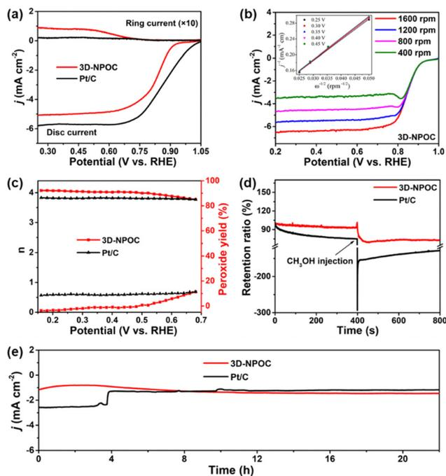
Fig. 3 (a) Polarization curves of 3D-NPOC and Pt/C are obtained at a scan rate of  $10 \text{ mV s}^{-1}$  in 0.1 M KOH electrolyte. (b) LSV curves of 3D-NPOC at varied rotation speeds from 400 to 1600 rpm. (c) Electron transfer numbers and the peroxide yields of 3D-NPOC and Pt/C at different potentials. (d) Chronoamperometric responses of 3D-NPOC and Pt/C at 0.7 V vs. RHE with 3 M  $\text{CH}_3\text{OH}$  added to the electrolyte. (e) Durability evaluation at 0.7 V vs. RHE of 3D-NPOC and Pt/C.
