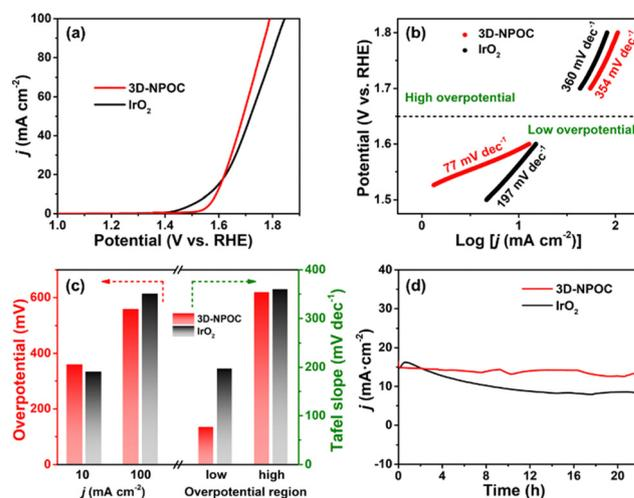
Fig. 4 (a) Polarization curves; (b) Tafel slopes derived from the corresponding polarization curves; (c) histogram of overpotentials at 10 and  $100 \text{ mA cm}^{-2}$ , and Tafel slopes at different overpotential regions; and (d) durability evaluation at a constant potential of 3D-NPOC and  $\text{IrO}_2$  for alkaline OER in 1.0 M KOH.
