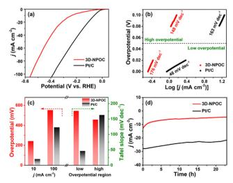
Fig. 5 (a) Polarization curves; (b) Tafel slopes derived from the corresponding polarization curves; (c) histogram of the overpotentials at 10 and 100 mA cm<sup>-2</sup>, and Tafel slopes at different overpotential regions; and (d) durability evaluation at a constant potential of 3D-NPOC and Pt/C for the alkaline HER in 1.0 M KOH
