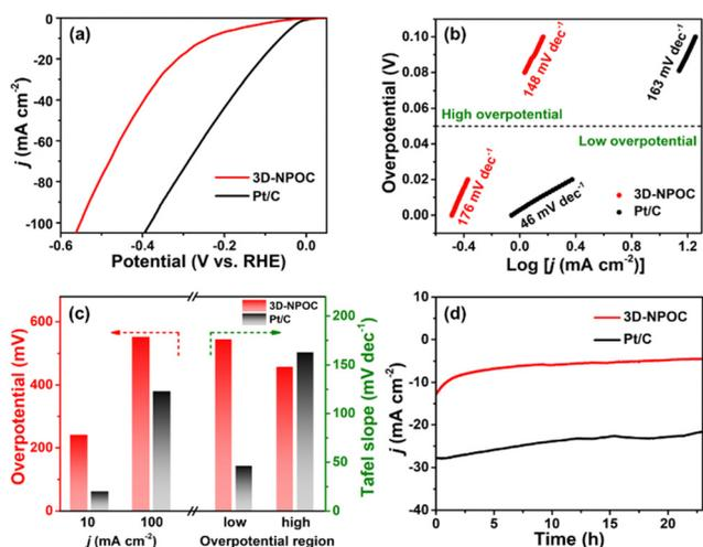
Fig. 5 (a) Polarization curves; (b) Tafel slopes derived from the corresponding polarization curves; (c) histogram of the overpotentials at 10 and  $100 \text{ mA cm}^{-2}$ , and Tafel slopes at different overpotential regions; and (d) durability evaluation at a constant potential of 3D-NPOC and Pt/C for the alkaline HER in 1.0 M KOH.
