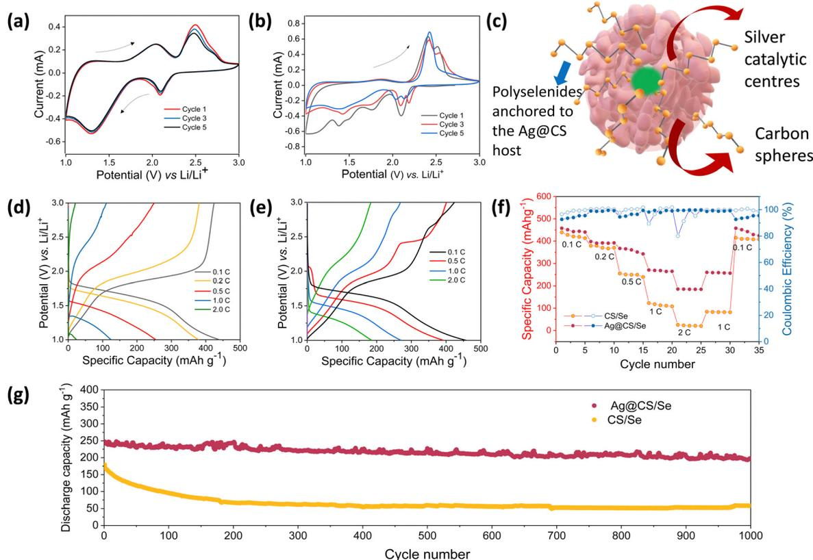
Fig. 3 CV profiles of Li–Se cells with (a) CS/Se and (b) Ag@CS/Se cathodes at 0.2 mV s<sup>-1</sup> sweep rate. (c) Schematic representation of the silver nano-reactors in CS. Cycling profiles of Li–Se cells with (d) CS/Se and (e) Ag@CS/Se cathodes recorded at different C-rates. Comparison of electrochemical performance in terms of (f) rate capability and (g) long cycling data at 1C rate (1000 cycles) for the CS/Se and Ag@CS/Se cathodes.
