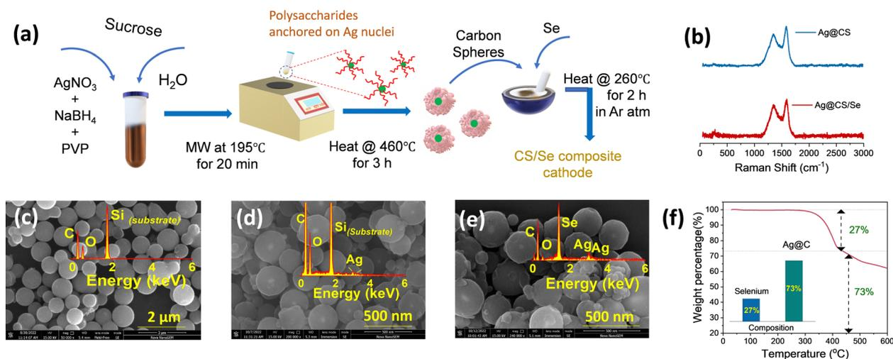
**Fig. 1** (a) Schematic representation of the microwave-assisted preparation of silver-centred CS and selenium incorporation. (b) Raman spectra of Ag@CS and Ag@CS/Se. SEM images of (c) carbon spheres, (d) Ag@CS and (e) selenium incorporated Ag@CS. The inset shows the respective EDX plots. (f) Estimation of selenium loading from TGA.
