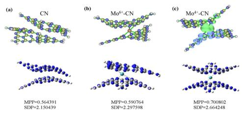
Fig. 7 The optimized structures (a) and spin density (b) of pristine CN, and Mo-doped CN.
