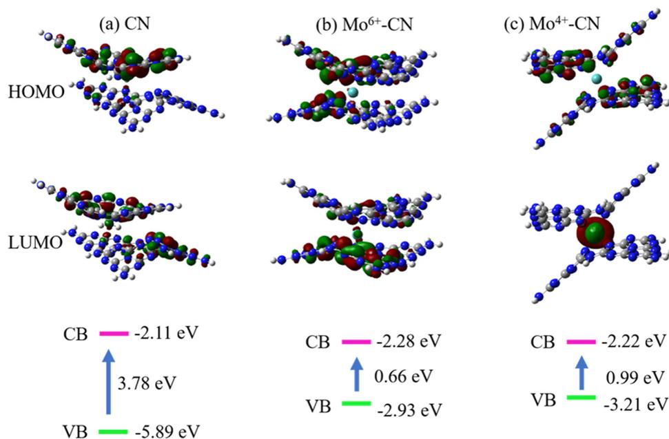
Fig. 8 HOMO, LUMO, and band gap of CN (a),  $\text{Mo}^{6+}$ -CN (b) and  $\text{Mo}^{4+}$ -CN (c). The iso-surface value is set at  $0.03 \text{ e bohr}^{-3}$ . Denotation: C atom – gray, N atom – dark blue.
