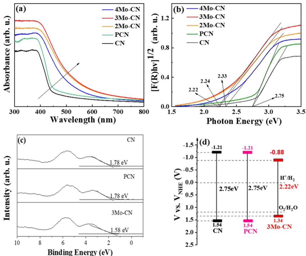
Fig. 4 UV-vis spectra (a), and the estimated band gaps (b) of CN, PCN, and Mo-doped CN. XPS valence band spectra (c), and schematic illustration of the band gap structure (d) of CN and 3Mo-CN.
