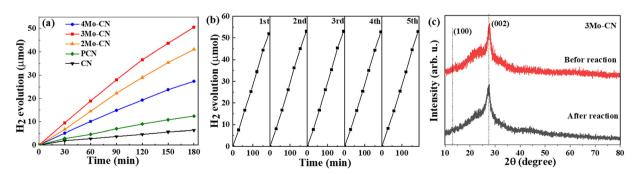
Fig. 6 Photocatalytic hydrogen evolution (a) of CN, PCN, and modoped CN. Stability test of 3Mo-CN (b). XRD patterns of 3Mo-CN before and after light irradiation (c)
