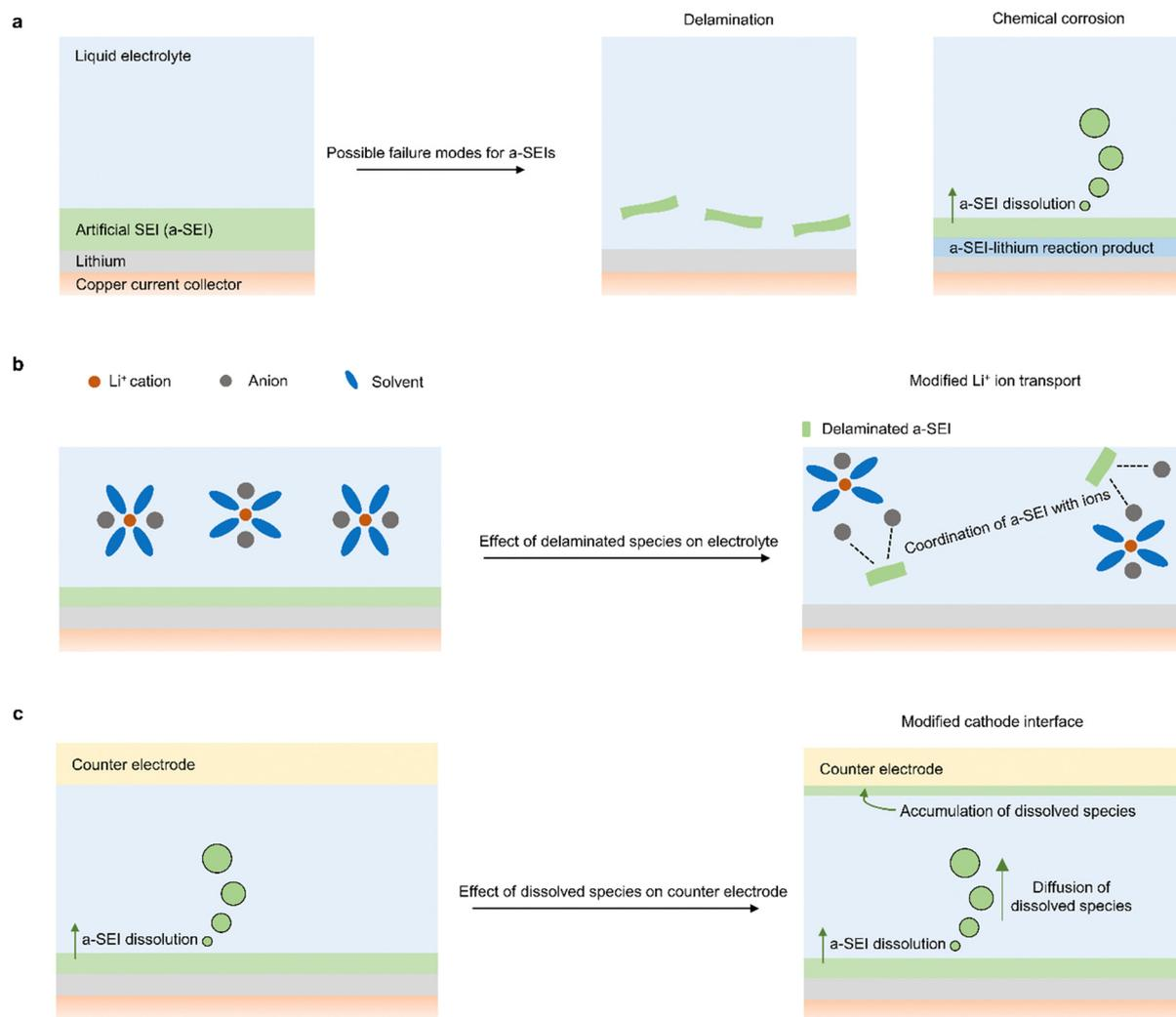
**Fig. 2** Design considerations for artificial SEIs: (a) illustration of possible failure modes of a-SEIs in lithium metal batteries. (b) Illustration of delaminated a-SEIs and their effects on ion transport. (c) Illustration of dissolved a-SEIs and their effects on counter electrodes.
