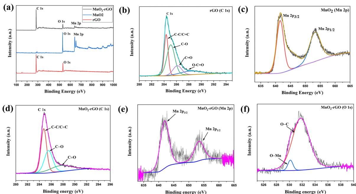
Fig. 3 (a) Full scan survey spectra of rGO, MnO<sub>2</sub> and the MnO<sub>2</sub>-rGO nanocomposite. The deconvoluted XPS spectrum of (b) rGO (C 1s) and (c) MnO<sub>2</sub> (Mn 2p). High-resolution XPS spectrum of (d) C 1s, (e) Mn 2p, and (f) O 1s of the MnO<sub>2</sub>-rGO nanocomposite.
