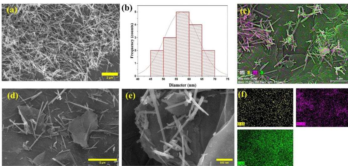
Fig. 1 (a) SEM image of the  $\text{MnO}_2$  nano-needles, (b)  $\text{MnO}_2$  nano-needles diameter size distribution, (d)–(e) FE-SEM image of the  $\text{MnO}_2$ -rGO nanocomposite, and (c) and (f)  $\text{MnO}_2$ -rGO nanocomposite elemental mapping.
