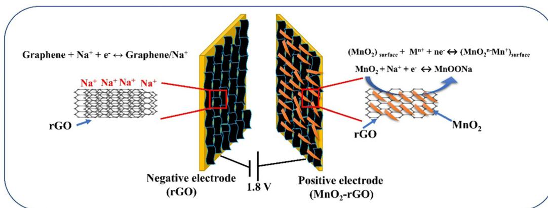
**Fig. 9** Charge storage mechanism of the wide 1.8 V voltage window quasi solid-state sodium ion ASC (rGO||MnO<sub>2</sub>-rGO) device.
