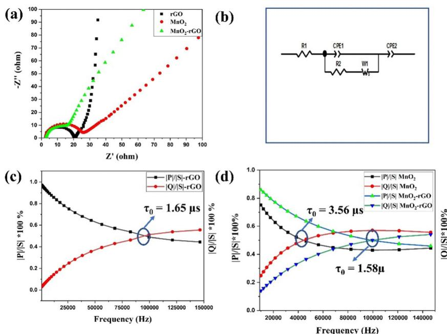
Fig. 7 (a) EIS spectra of rGO,  $\text{MnO}_2$  and the  $\text{MnO}_2$ -rGO electrode, (b) equivalent fitted circuit of the EIS data. Plot between  $|P|/|S|$  and  $|Q|/|S|$  along with frequency (Hz) for the (c) rGO-electrode and (d)  $\text{MnO}_2$  and  $\text{MnO}_2$ -rGO-electrode.
