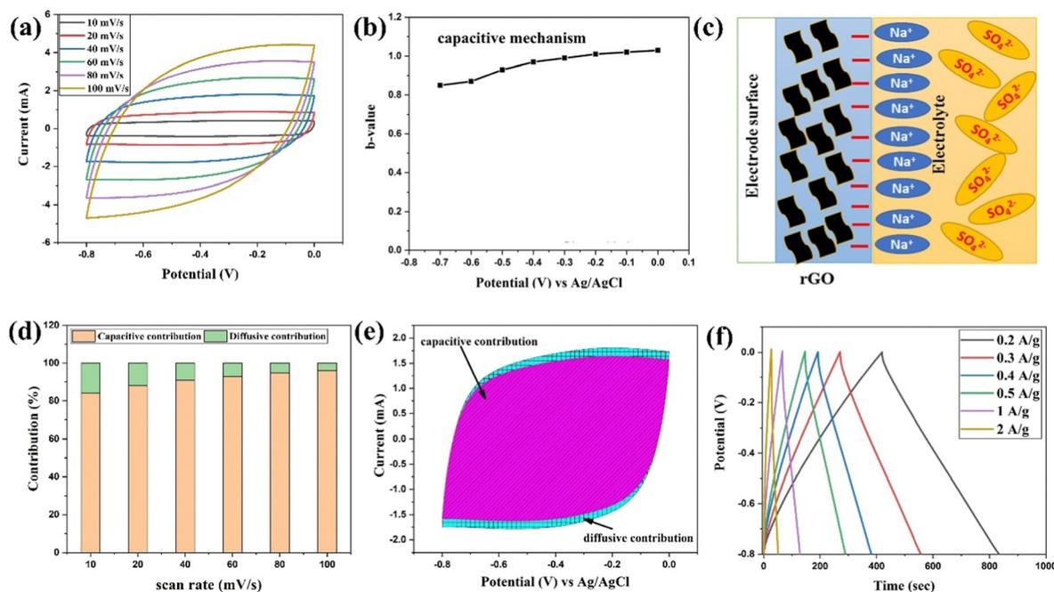
Fig. 5 (a) CV profile of the rGO-electrode at several sweep rates. (b) Variation of the  $b$  value at various applied voltages. (c) Graphical illustration of the charge storage in the rGO electrode. (d) Percentage capacitive and diffusive contribution as the function of scan rates of the rGO-electrode. (e) CV curve of the rGO electrode (at  $40 \text{ mV s}^{-1}$ ) and (f) GCD curve for the rGO electrode at different current densities.
