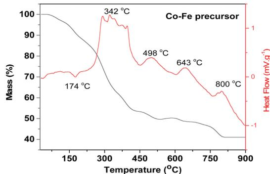
Fig. 2 Thermogravimetric (TGA) curve for the Co-Fe precursor.
