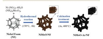
Fig. 1 Schematic illustration of the synthesis process of the NiMoO-Ar/NF
