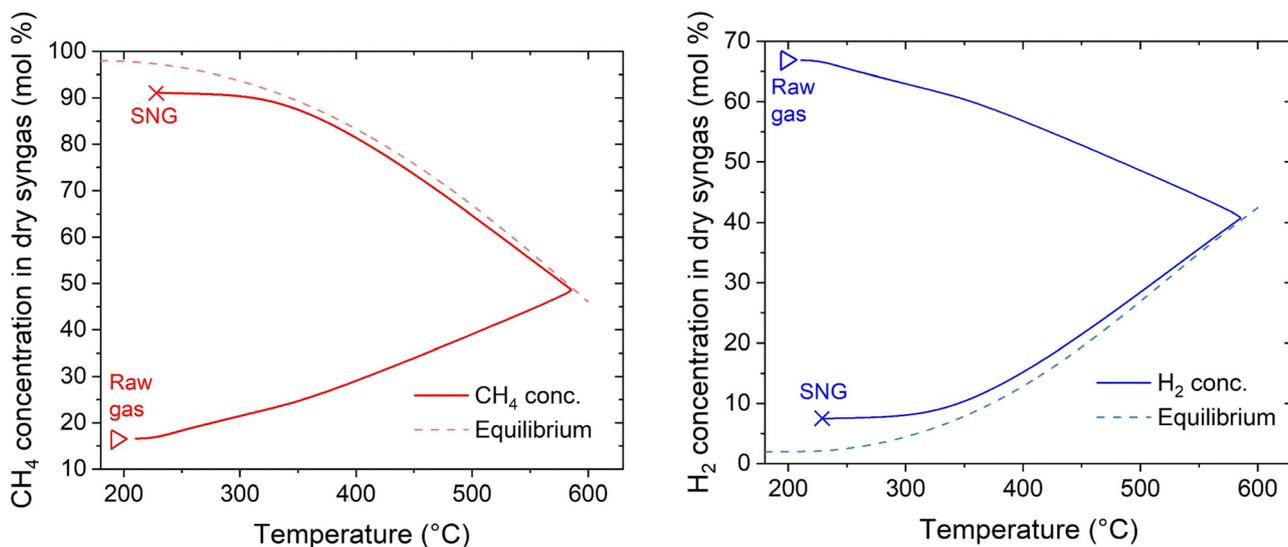
Fig. 10 Calculated concentration profiles in the reactor as a function of temperature (experimental conditions: 8 bar, H<sub>2</sub>:CO<sub>2</sub> = 4.15, CO<sub>2</sub>:CH<sub>4</sub> = 1:1, cooling setpoint = 230 °C, load = 100%).
