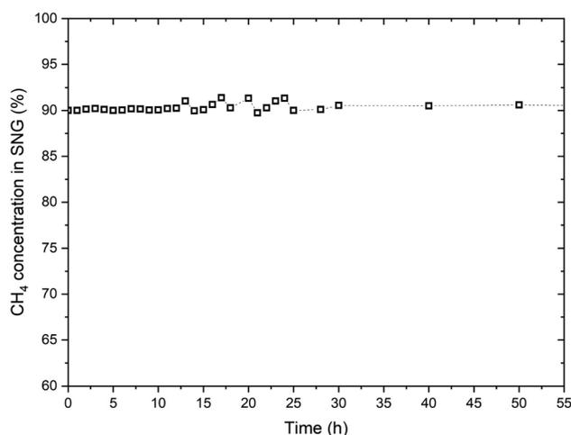
Fig. 11 The CH<sub>4</sub> concentration in SNG over the first 50 hours of operation of the reactor.
