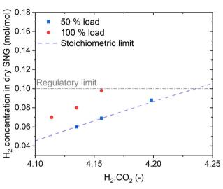
Fig. 4 The effect of stoichiometric ratio on the H<sub>2</sub> concentration in the SNG (experimental conditions: 8 bar, cooling setpoint = 230 °C).
