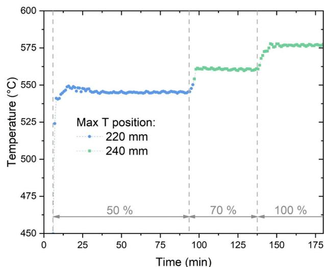
Fig. 3 The evolution of the maximum temperature in the methanation reactor (experimental conditions: 8 bar, H<sub>2</sub>:CO<sub>2</sub> = 4.15, cooling setpoint = 230 °C).
