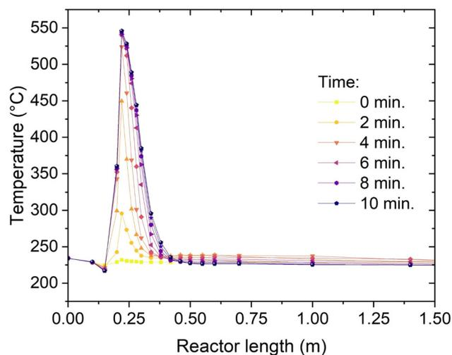
Fig. 7 Temperature profile at the start-up (experimental conditions: 8 bar, H<sub>2</sub>:CO<sub>2</sub> = 4.15, cooling set point = 230 °C).
