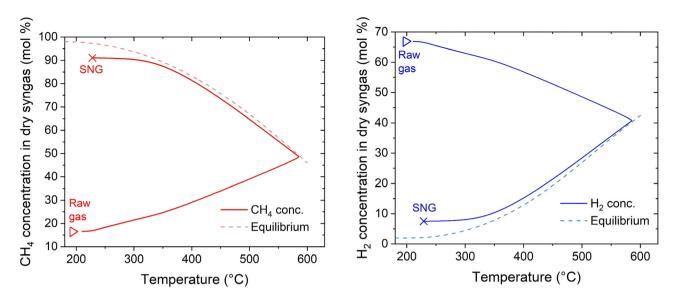
Fig. 10 Calculated concentration profiles in the reactor as a function of temperature (experimental conditions: 8 bar,  $H_2$ :  $CO_2$  = 4.15,  $CO_2$ :  $CH_4$  = 1:1, cooling setpoint = 230 °C, load = 100%).
