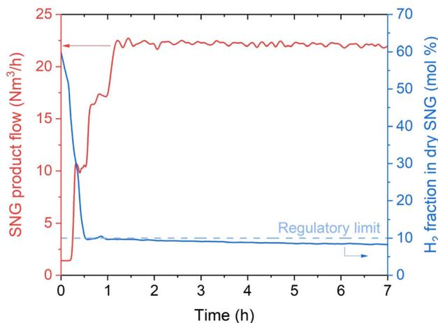
Fig. 2 Productivity and H<sub>2</sub> fraction in SNG at the reactor outlet at the start-up of the biogas methanation plant (experimental conditions: 8 bar, H<sub>2</sub>:CO<sub>2</sub> = 4.15, cooling setpoint = 230 °C). The CO<sub>2</sub> conversion is 100% in the entire time interval considered and no other products than methane were observed.
