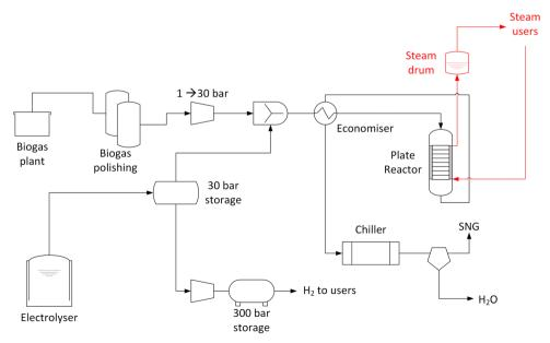
Fig. 1 Schematic representation of the installed biogas methanation plant.
