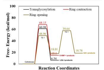
Fig. 1 Gas phase activation free energy barriers for cellobiose decomposition calculated using hybrid functional M06-2X with 6-311+G(d) basis set for transglycosylation, ring contraction and ring opening mechanisms.
