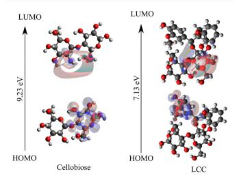
Fig. 3 HOMO-LUMO orbitals are visualized using frontier orbital analysis performed on isolated cellobiose and cross-linked cellobiose in LCC.
