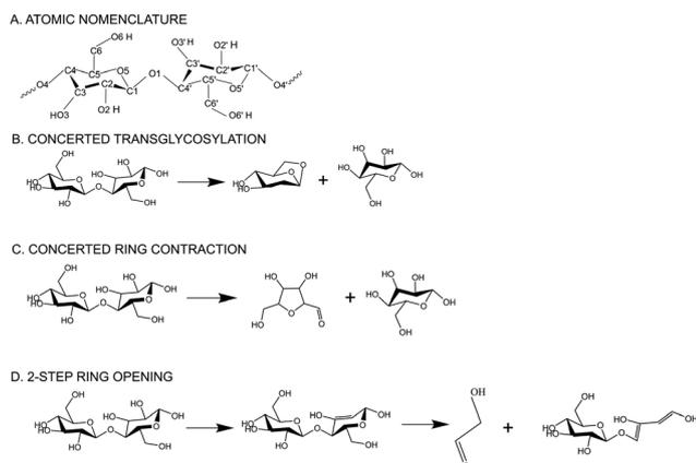
**Scheme 1** (A) Atomic nomenclature of the monomeric glucose unit (B) transglycosylation reaction mechanism of cellobiose decomposition to form LGA (C) ring contraction mechanism of cellobiose decomposition to form furanic compounds (D) ring opening mechanism of cellobiose decomposition to form glycolaldehyde.
