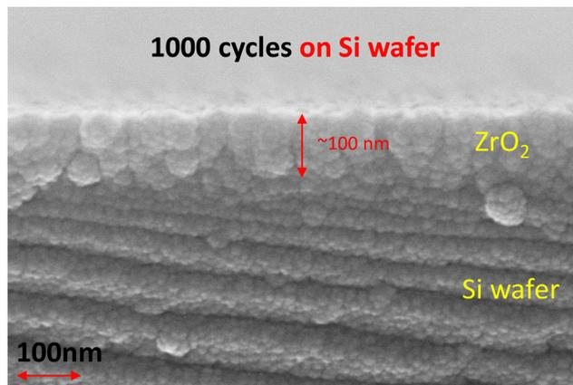
Fig. 1 SEM image of the cross-section of an ALD-ZrO<sub>2</sub>@Si.
