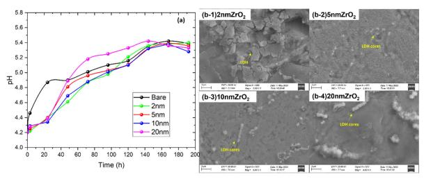
Fig. 3 (a) pH change in 2 M ZnSO<sub>4</sub> soaked with bare Zn and 2–20 nm ALD-ZrO<sub>2</sub>@Zn and (b-1)–(b-4) SEM images of ALD-ZrO<sub>2</sub>@Zn surface after soaking in 2 M ZnSO<sub>4</sub> for 200 h.
