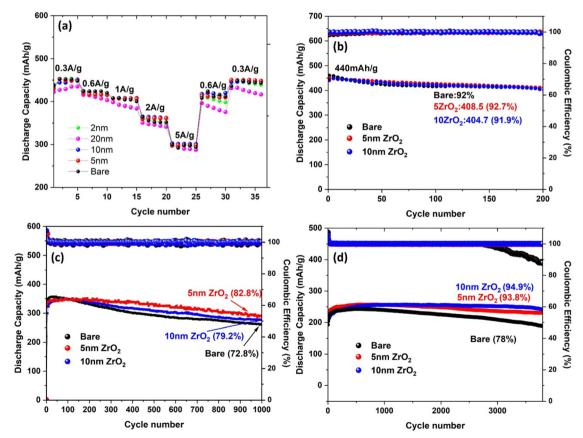
Fig. 7 Stability of ZnVO|2 M ZnSO<sub>4</sub>|ALD-ZrO<sub>2</sub>@Zn full batteries at (a) different rates of 0.3–5 A  $g^{-1}$ , (b) low 0.3 A  $g^{-1}$ , (c) medium 2 A  $g^{-1}$  and (d) high 10 A  $g^{-1}$ .
