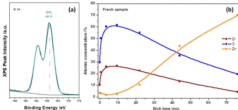
Fig. 2 XPS spectra of (a) Zr 3d and (b) depth profiling of Zr and O in an as-deposited 10 nm ALD-ZrO<sub>2</sub>@Zn.
