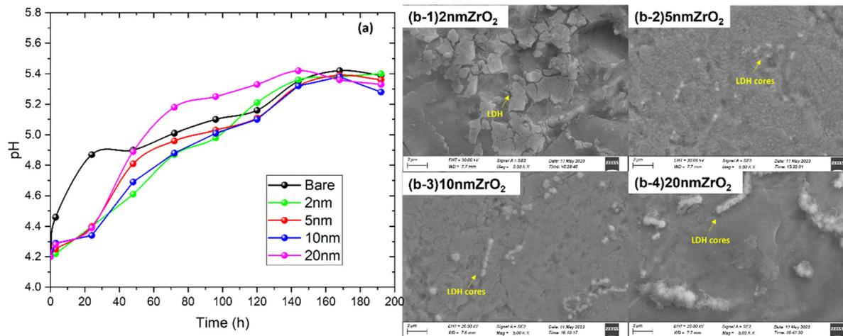
Fig. 3 (a) pH change in 2 M ZnSO<sub>4</sub> soaked with bare Zn and 2–20 nm ALD-ZrO<sub>2</sub>@Zn and (b-1)–(b-4) SEM images of ALD-ZrO<sub>2</sub>@Zn surface after soaking in 2 M ZnSO<sub>4</sub> for 200 h.
