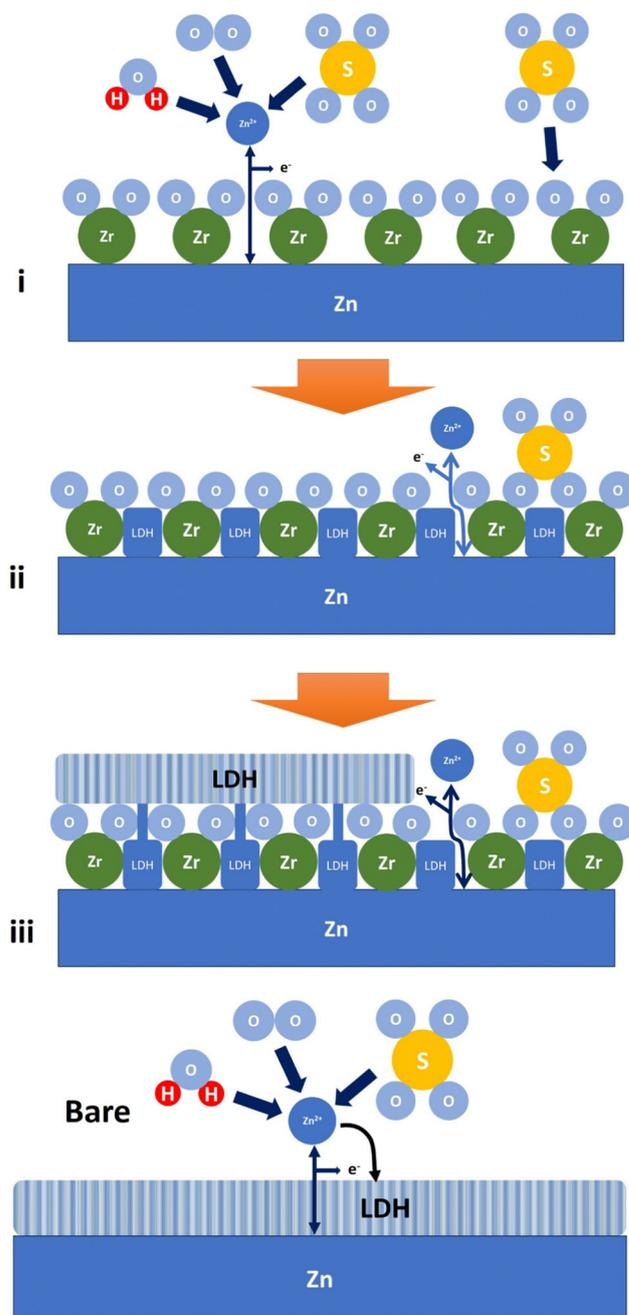
Fig. 8 A schematic illustrating the formation of Zn-LDH on ALD-ZrO<sub>2</sub>@Zn and bare Zn. Label (i)–(iii) refers to stage 1–3 as discussed, respectively.
