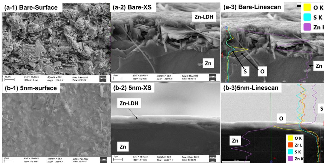
Fig. 6 SEM analysis of Zn electrode after symmetrical cell tests. (a) Bare Zn; and (b) 5 nm ALD-ZrO<sub>2</sub>@Zn.
