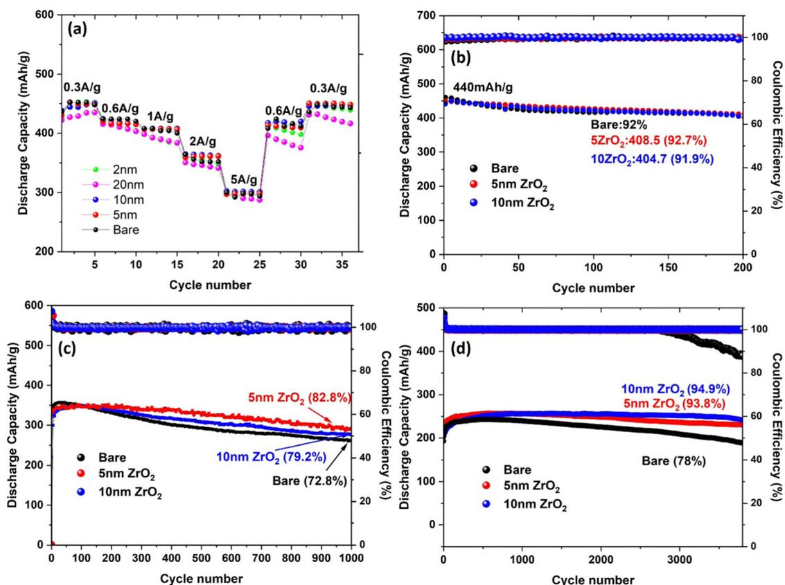
Fig. 7 Stability of ZnVO|2 M ZnSO<sub>4</sub>|ALD-ZrO<sub>2</sub>@Zn full batteries at (a) different rates of 0.3–5 A g<sup>-1</sup>, (b) low 0.3 A g<sup>-1</sup>, (c) medium 2 A g<sup>-1</sup> and (d) high 10 A g<sup>-1</sup>.
