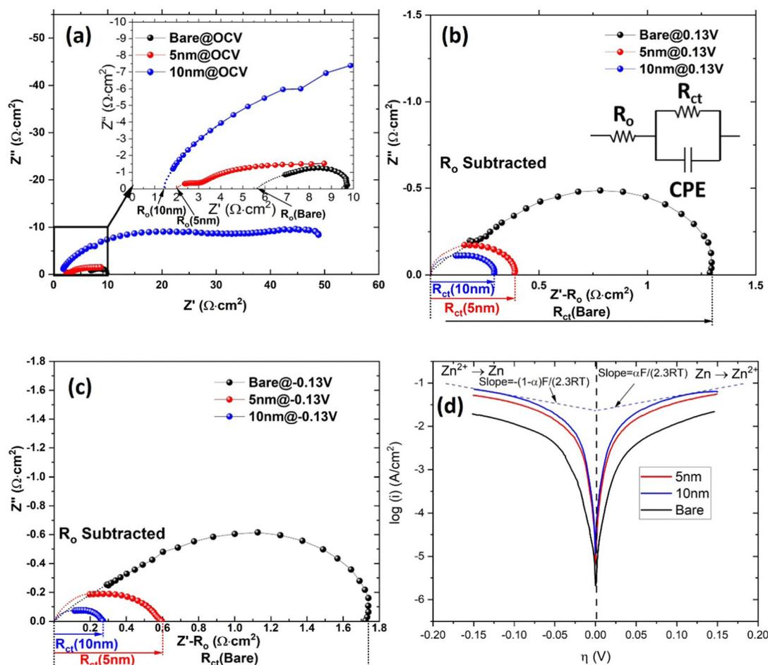
Fig. 4 EIS spectra under (a) OCV, (b) 0.13 V bias and (c) -0.13 V bias and (d) Tafel plots from potential dynamics of 3-electrode cell using uncoated and ALD-ZrO<sub>2</sub>@Zn as working electrode. ALD-ZrO<sub>2</sub> thickness: 5 and 10 nm. Note that  $R_o$  was subtracted from EIS spectra in (b) and (c).
