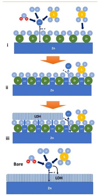
Fig. 8 A schematic illustrating the formation of Zn-LDH on ALD-ZrO2@Zn and bare Zn. Label (i)-(iii) refers to stage 1-3 as discussed, respectively.
