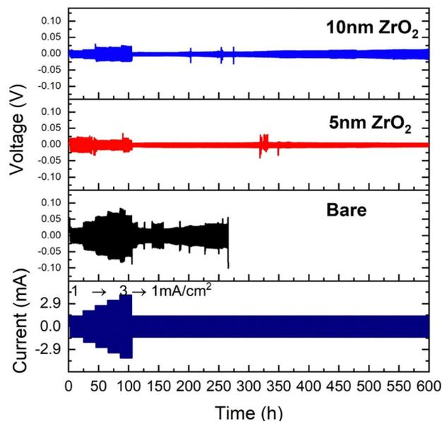
**Fig. 5** Cycling stability of symmetrical coin cells at ±1 to ±3 mA cm<sup>-2</sup> with 2 M ZnSO<sub>4</sub>/glass fiber as electrolyte and bare Zn, and 5 nm and 10 nm ALD-ZrO<sub>2</sub>@Zn as electrodes.
