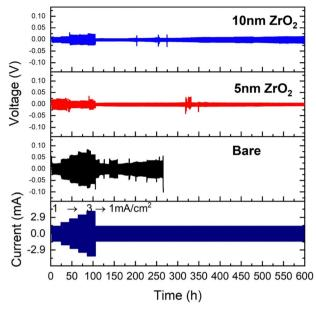
Fig. 5 Cycling stability of symmetrical coin cells at  $\pm 1$  to  $\pm 3$  mA cm-2with 2 M ZnSO<sub>4</sub>/glass fiber as electrolyte and bare Zn, and 5 nm and 10 nm ALD-ZrO2@Zn as electrodes.
