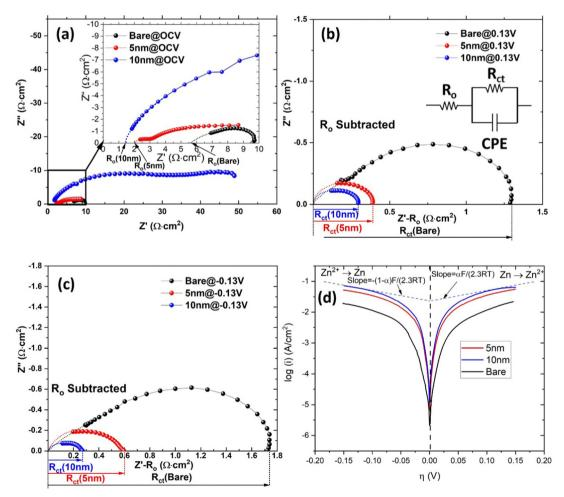
Fig. 4 EIS spectra under (a) OCV, (b) 0.13 V bias and (c) -0.13 V bias and (d) Tafel plots from potential dynamics of 3-electrode cell using uncoated and ALD-ZrO<sub>2</sub>@Zn as working electrode. ALD-ZrO<sub>2</sub> thickness: 5 and 10 nm. Note that  $R_0$  was subtracted from EIS spectra in (b) and (c).
