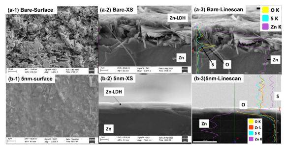
Fig. 6 SEM analysis of Zn electrode after symmetrical cell tests. (a) Bare Zn; and (b) 5 nm ALD-ZrO<sub>2</sub>@Zn.
