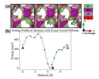
Fig. 9 Li vacancy evolution of the cross-tunnel pathway (PathwayII) in the vacancy limit. (a) Shows images along the pathway, where dashed circles indicate positions of vacancies; vacancy positions labeled  $\alpha_1$ ,  $\beta_2$  and  $\alpha_3$ have the same positions with identical labels in Fig. 4. (b) Shows calculated energy evolution as a function of vacancy migration distance, where labels  $\alpha_1$ ,  $\beta_2$  and  $\alpha_3$  correspond to the images in (a).
