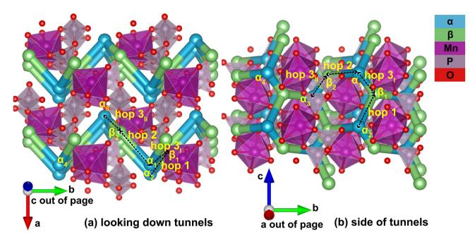
Fig. 4 Connectivity between meta-stable sites as constructed by MigrationGraph, where (a) shows tunnels going in and out of page, and (b) shows tunnels going up and down, along the direction of lattice vector c. Neighboring meta-stable sites, labeled  $\alpha$  and  $\beta$  based on symmetry, are connected via hops shown as cylinders. Sites and hops with identical labels in (a) and (b) are identical.
