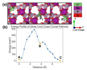
Fig. 7 Li-ion evolution of the along-tunnel pathway (PathwayII) in the dilute limit. (a) Shows images along the pathway, and Li positions labeled  $\alpha_1$ ,  $\beta_2$  and  $\alpha_3$  have the same positions with identical labels in Fig. 4. (b) Shows calculated energy evolution as a function of Li migration distance, where labels  $\alpha_1$ ,  $\beta_2$  and  $\alpha_3$  correspond to the images in (a).
