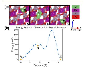
Fig. 6 Li-ion evolution of the along-tunnel pathway (Pathwayl) in the dilute limit. (a) Shows images along the pathway, and Li positions labeled  $\alpha_1$ ,  $\beta_1$  and  $\alpha_2$  have the same positions with identical labels in Fig. 4. (b) Shows calculated energy evolution as a function of Li migration distance, where labels  $\alpha_1$ ,  $\beta_1$  and  $\alpha_2$  correspond to the images in (a).
