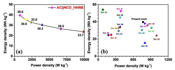
Fig. 6 (a) The Ragone plot showing power and energy density at different current densities and (b) comparison of the present work with some of the recent results published on NiCo<sub>2</sub>O<sub>4</sub> (including composites) as the host material.
