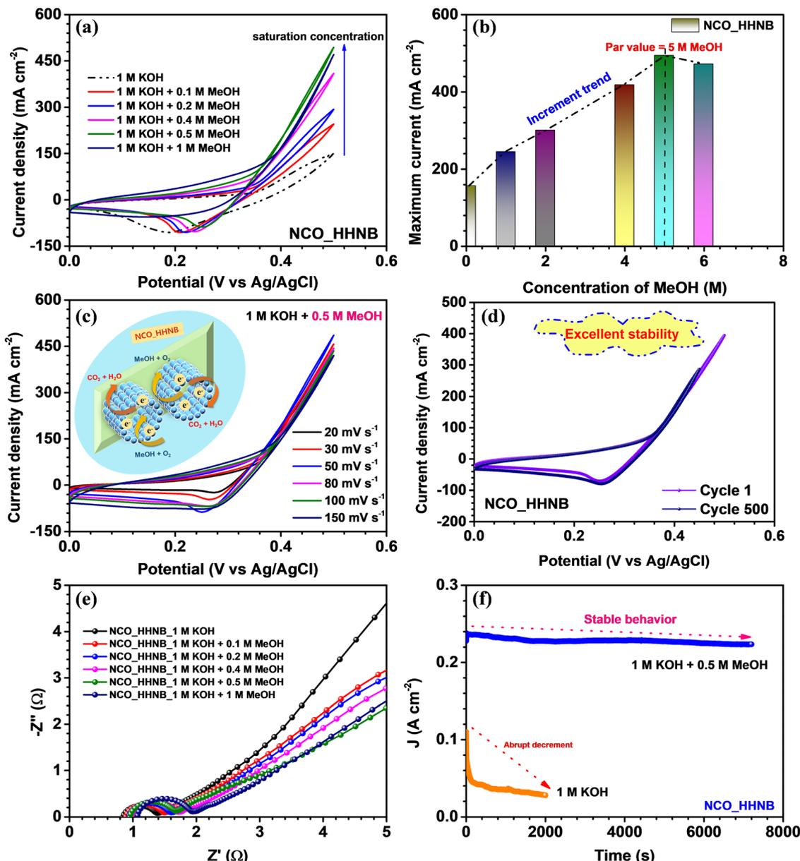
Fig. 7 (a) CV profiles at various scan rates, (b) change in the anodic current, (c) EIS profiles at different concentrations of MeOH in KOH, (d) CV profiles at different scan rates in 0.5 M MeOH + 1 M KOH electrolytic system, (e) comparative cyclic voltammograms at 50 mV s<sup>-1</sup> of cycles 1 and 500 and (f) chronoamperometric tests to check the stability of the NCO\_HHNB electrode in 0.5 M MeOH + 1 M KOH and bare KOH electrolytes.
