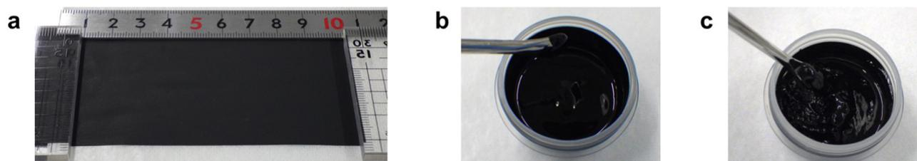
Fig. 3 (a) Photographic image of the electrode of  $\text{Li}_2\text{RuO}_3/\text{Li}_2\text{SO}_4$  with a  $\text{Li}_2\text{SO}_4$  ratio of 0.24 and with a mass loading of 20  $\text{mg cm}^{-2}$ . (b) and (c) Photographic image of slurry solution of  $\text{Li}_2\text{RuO}_3/\text{Li}_2\text{SO}_4$  with  $\text{Li}_2\text{SO}_4$  ratios of (b) 0.24 and (c) 0.1.
