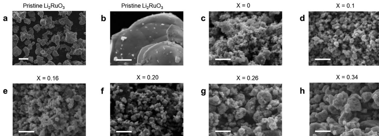
Fig. 2 SEM-EDS images of (a) and (b) pristine  $\text{Li}_2\text{RuO}_3$  and (c)–(h)  $\text{Li}_2\text{RuO}_3/\text{Li}_2\text{SO}_4$  samples. Scale bars are (a) 10  $\mu\text{m}$  and (b)–(h) 1  $\mu\text{m}$ .
