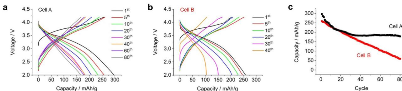
Fig. 5 (a) and (b) Charge/discharge profile of the electrochemical cell equipped with the  $\text{Li}_2\text{RuO}_3/\text{Li}_2\text{SO}_4$  sample ( $x = 0.2$ ) as the positive electrode: (a) cell A and (b) cell B. (c) Discharge capacity plotted against the cycle number for cell A (black curve) and cell B (red curve).
