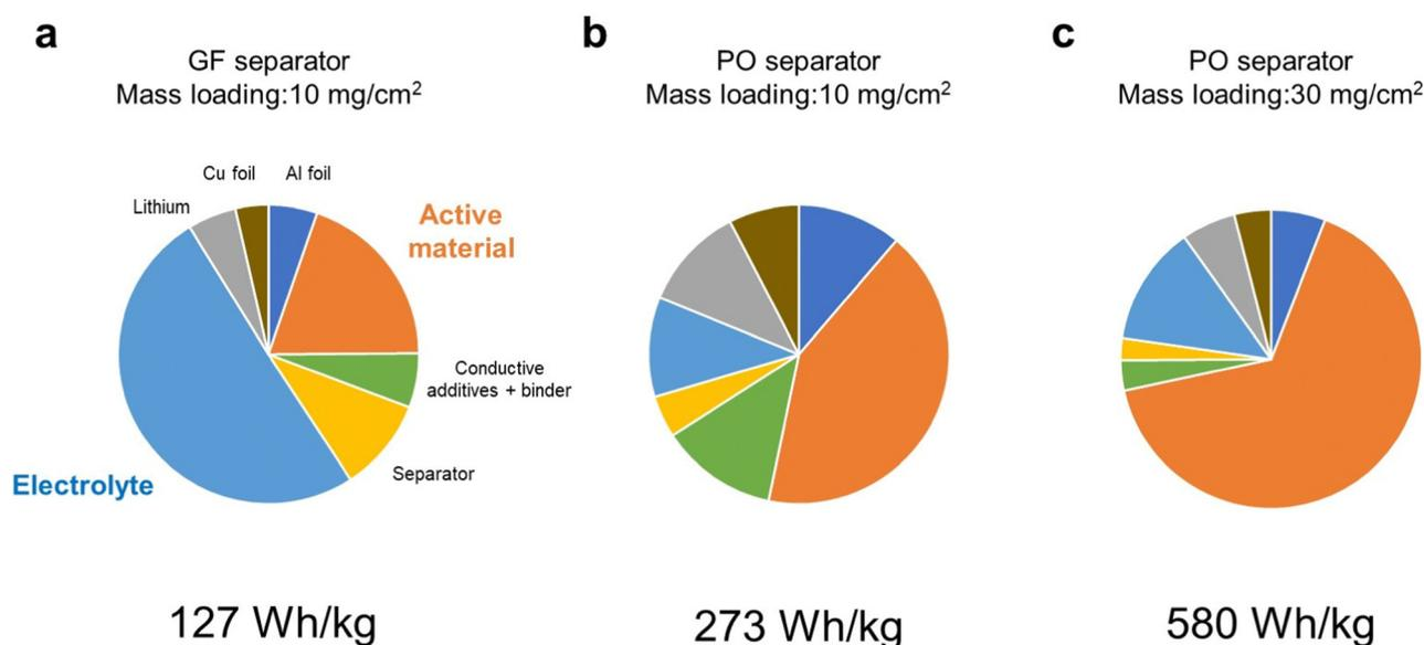
Fig. 1 Weight fractions of LMB components calculated using the parameters listed in Table S1 (ESI<sup>†</sup>). (a) Glass fiber separator, a mass loading of 10 mg cm<sup>-2</sup>, (b) polyolefin separator, a mass loading of 10 mg cm<sup>-2</sup>, and (c) polyolefin separator, a mass loading of 30 mg cm<sup>-2</sup>.
