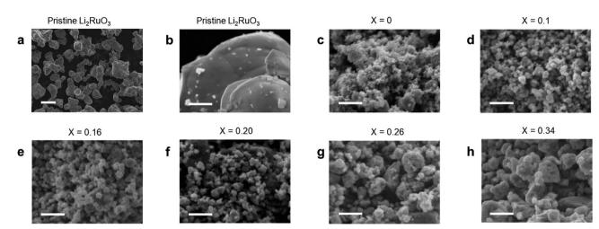
SEM-EDS images of (a) and (b) pristine  $\text{Li}_2\text{RuO}_3$  and (c)-(h)  $\text{Li}_2\text{RuO}_3/\text{Li}_2\text{SO}_4$  samples. Scale bars are (a) 10  $\mu$ m and (b)-(h) 1  $\mu$ m.
