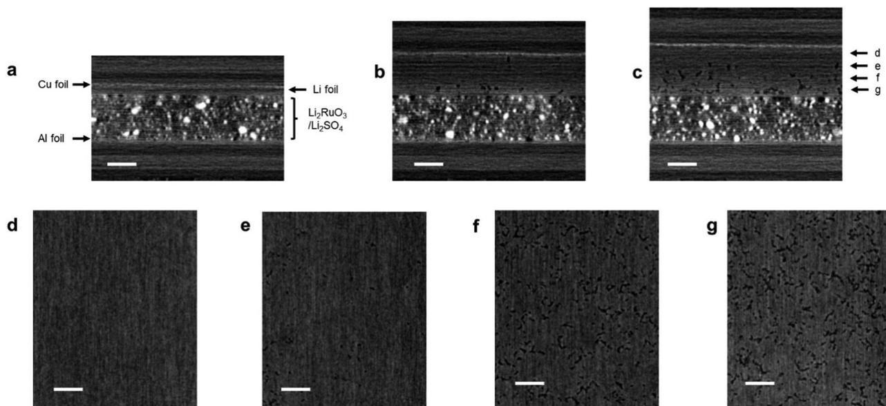
Fig. 6 (a)–(c) X-ray CT images of cell B; (a) as prepared, (b) after the 10th cycle, and (c) after the 20th cycle in the cross-sectional direction; (d)–(g) X-ray CT images of cell B after the 20th cycle in the surface direction. Scale bars are  $100 \mu\text{m}$ .
