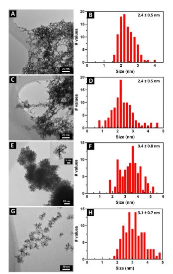
Fig. 1 TEM images and size distributions are shown of a range of chemically distinctive ultrathin NWs, prepared by different synthesis methods. (A) and (B) Pt<sub>1</sub>Ru<sub>1</sub> and (C) and (D) Pt<sub>3</sub>Ru<sub>1</sub> were both prepared with CTAB. (E) and (F) Pt<sub>1</sub>Ru<sub>1</sub> with the inset showing an individual cluster as well as (G) and (H) Pt<sub>1</sub>Ru<sub>9</sub> were generated with OAm and OA.
