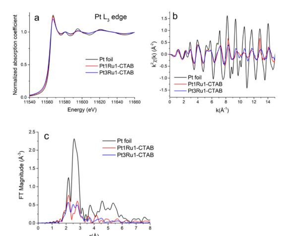
Fig. 4 (A) Pt  $L_3$ -edge XANES data. (B)  $k^2$ -weighted EXAFS data in k-space. (C) Fourier transform magnitudes of the  $k^2$ -weighted EXAFS data for Pt foil, Pt<sub>1</sub>Ru<sub>1</sub> (produced with CTAB), and Pt<sub>3</sub>Ru<sub>1</sub> (produced with CTAB).
