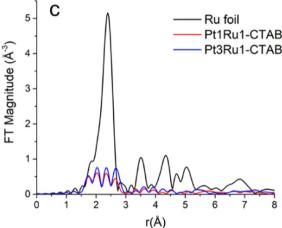
(A) Ru K-edge XANES data. (B)  $k^2$ -weighted EXAFS data in k-space. (C) Fourier transform magnitudes of the  $k^2$ -weighted EXAFS data for Ru foil, Pt<sub>1</sub>Ru<sub>1</sub> (produced with CTAB), and Pt<sub>3</sub>Ru<sub>1</sub> (generated with CTAB).
