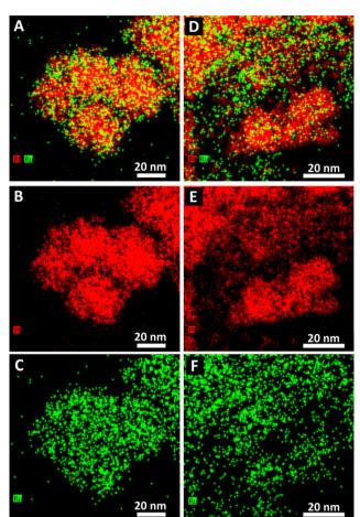
Fig. 3 EDS elemental maps of PtRu prepared using the OAm/OA method.  $Pt_1Ru_1$  maps are given as (A) the composite of Pt and Ru, (B) Pt, and (C) Ru. Corresponding Pt<sub>1</sub>Ru<sub>9</sub> elemental maps are shown in (D) the composite of Pt and Ru, (E) Pt, and (F) Ru.
