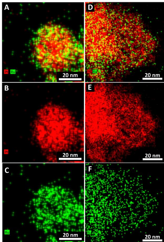
Fig. 2 EDS elemental maps of PtRu generated using the CTAB method.  $\text{Pt}_1\text{Ru}_1$  maps are provided as follows: (A) the composite of Pt and Ru, (B) Pt, and (C) Ru. Analogous  $\text{Pt}_3\text{Ru}_1$  maps are shown, as (D) the composite of Pt and Ru, (E) Pt, and (F) Ru.
