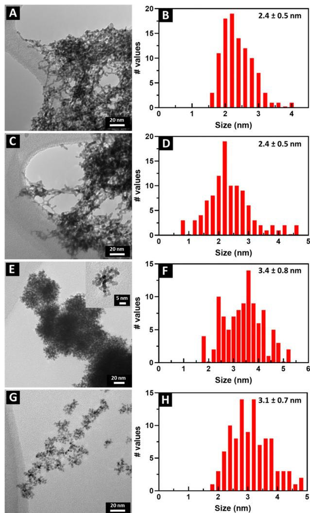
Fig. 1 TEM images and size distributions are shown of a range of chemically distinctive ultrathin NWs, prepared by different synthesis methods. (A) and (B)  $\text{Pt}_1\text{Ru}_1$  and (C) and (D)  $\text{Pt}_3\text{Ru}_1$  were both prepared with CTAB. (E) and (F)  $\text{Pt}_1\text{Ru}_1$  with the inset showing an individual cluster as well as (G) and (H)  $\text{Pt}_1\text{Ru}_9$  were generated with OAm and OA.
