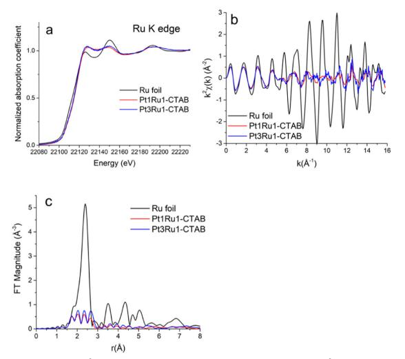
(A) Ru K-edge XANES data. (B)  $k^2$ -weighted EXAFS data in k-space. (C) Fourier transform magnitudes of the  $k^2$ -weighted EXAFS data for Ru foil, Pt<sub>1</sub>Ru<sub>1</sub> (produced with CTAB), and Pt<sub>3</sub>Ru<sub>1</sub> (generated with CTAB).
