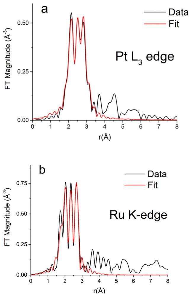
Fig. 6 Fourier transform magnitudes of  $k^2$ -weighted EXAFS data and theoretical fits for the  $\text{Pt}_3\text{Ru}_1$  (generated with CTAB) sample at (A) the  $\text{Pt}$   $L_3$ -edge and (B) the  $\text{Ru}$   $K$ -edge.
