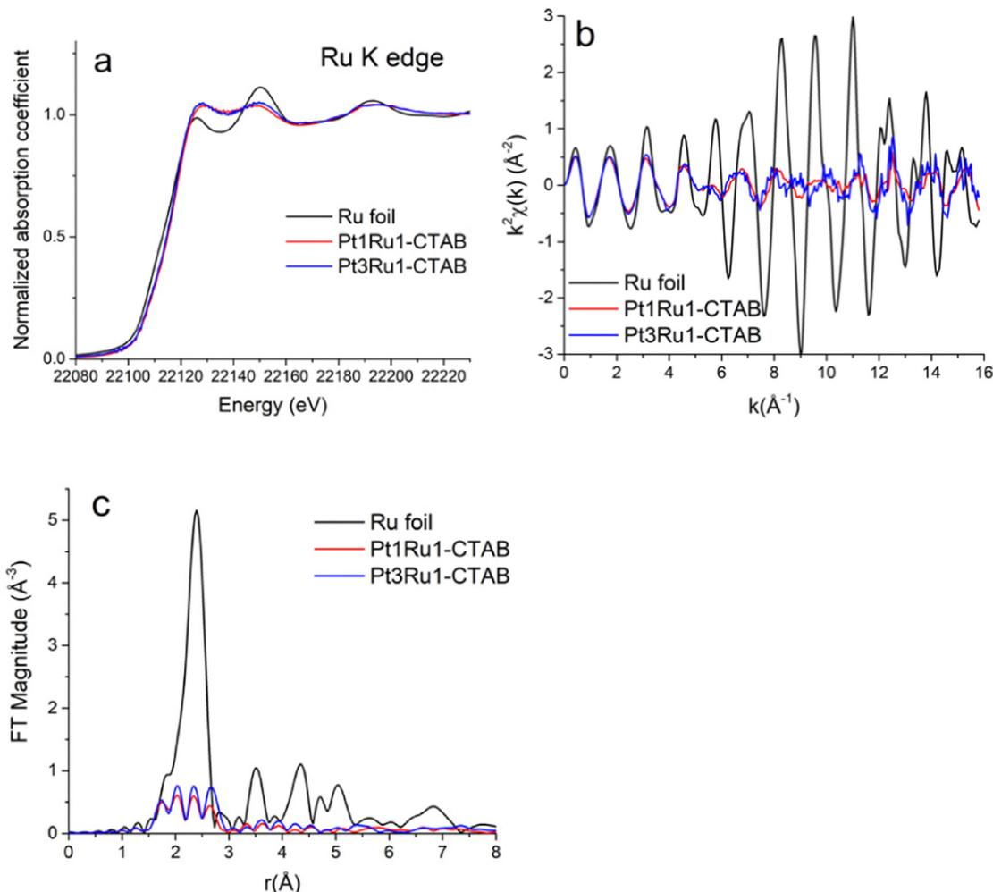
Fig. 5 (A) Ru K-edge XANES data. (B)  $k^2$ -weighted EXAFS data in  $k$ -space. (C) Fourier transform magnitudes of the  $k^2$ -weighted EXAFS data for Ru foil, Pt<sub>1</sub>Ru<sub>1</sub> (produced with CTAB), and Pt<sub>3</sub>Ru<sub>1</sub> (generated with CTAB).
