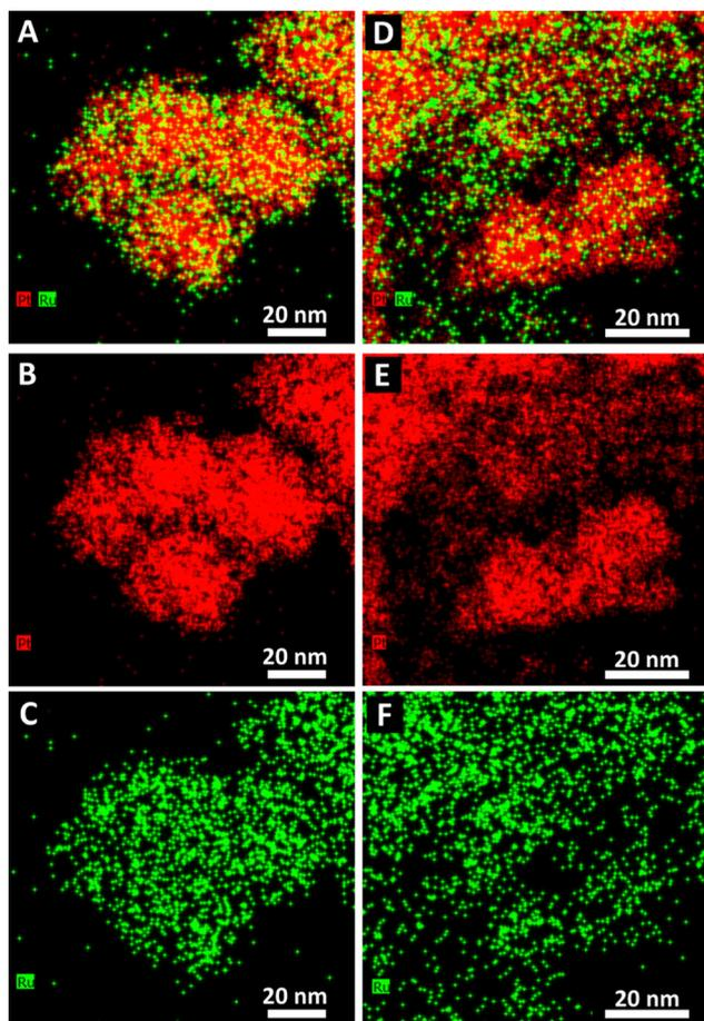
Fig. 3 EDS elemental maps of PtRu prepared using the OAm/OA method. Pt<sub>1</sub>Ru<sub>1</sub> maps are given as (A) the composite of Pt and Ru, (B) Pt, and (C) Ru. Corresponding Pt<sub>1</sub>Ru<sub>9</sub> elemental maps are shown in (D) the composite of Pt and Ru, (E) Pt, and (F) Ru.
