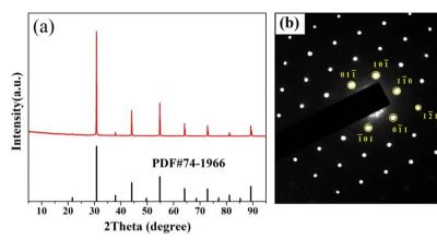
Fig. 1 (a) XRD pattern and (b) SAED pattern of BaTa<sub>0.5</sub>Li<sub>0.5</sub>O<sub>2.5</sub>
