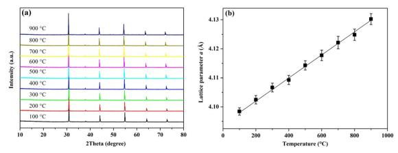
Fig. 3 (a) VT-XRD patterns and (b) corresponding lattice parameters of BTLO.
