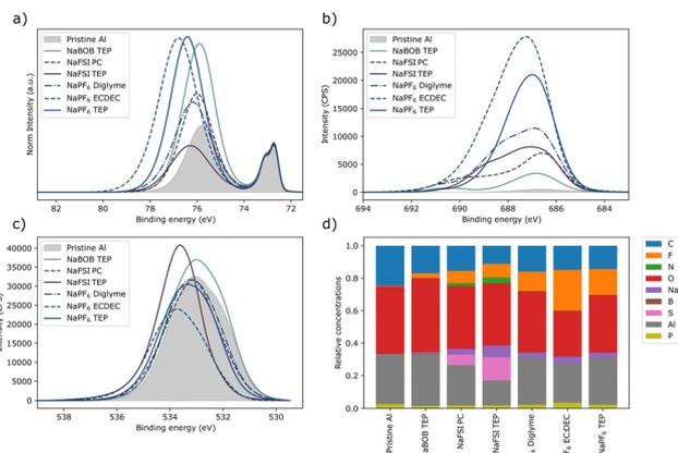
**Fig. 4** XPS deconvolution results of the spectra shown in Fig. S6–S8 (ESI<sup>†</sup>). The spectra shown here are energy calibrated to the “bulk”-signal of aluminum Al2p positioned to 72.7 eV, (a) Al2p, (b) F1s, and (c) O1s core levels. The relative atomic concentrations are shown in (d), this estimation is based on the models in Fig. S6–S8 (ESI<sup>†</sup>). The spectra in (a) have been area normalized to the intensity that was believed to be caused by the pure aluminium (“bulk” aluminium).
