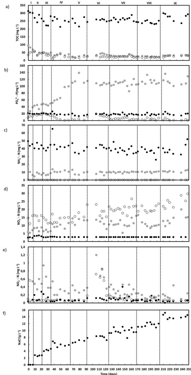
Fig. 1 TOC (a), phosphate (b), ammonium (c), nitrate (d), nitrite (e) and salt (f) concentrations along AGS-reactor operation. Concentration in the wastewater (●), in the reactor bulk liquid after anaerobic feeding (●) and outlet (○) are shown.
