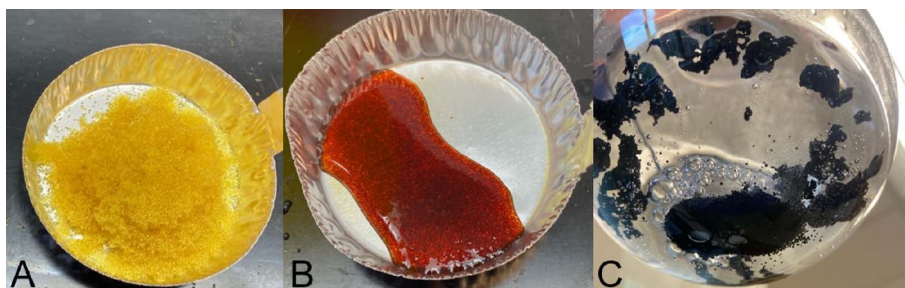
Fig. 3 Key failed NZVI-A600E synthesis outcomes: (A) A600E after \text{FeCl}_4^- loading with 20% ethanol and no HCl, (B) \text{FeCl}_4^- -A600E after rinsing with water until pH = 7, forming \text{Fe}(\text{OH})_3(\text{s}) , (C) NZVI-A600E and NZVI in bulk solution due to lack of \text{FeCl}_4^- -A600E rinsing in ethanol.
