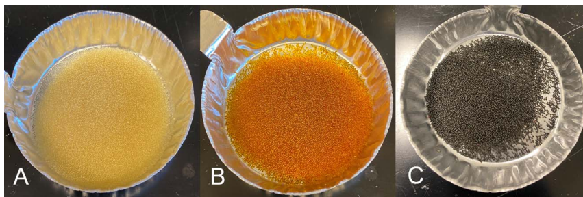
Fig. 2 Photographs of resin at different synthesis steps, including (A) pristine A600E (B) \text{FeCl}_4^- -A600E (C) NZVI-A600E.
