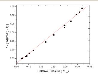
Fig. 4 Adsorption–desorption plot of  $N_2$  at 77.35 K for baobab seed-derived biochar.
