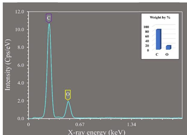
Fig. 2 The EDX micrograph illustrates the existence of carbon and oxygen in the biochar derived from baobab seeds after pyrolysis at 700 °C.
