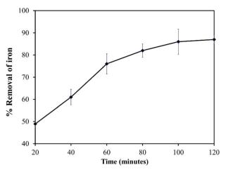
Fig. 6 Effect of contact time on % removal of Fe from aqueous solution.
