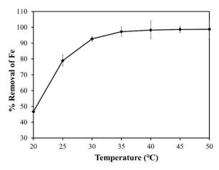
Fig. 9 Effect of solution temperature on Fe removal from groundwater.
