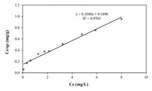
Fig. 11 The Langmuir isotherm plot for Fe removal using baobab seed-derived biochar (adsorbent).
