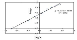
Fig. 12 The Freundlich isotherm plot for Fe removal using baobab seed-derived biochar (adsorbent).
