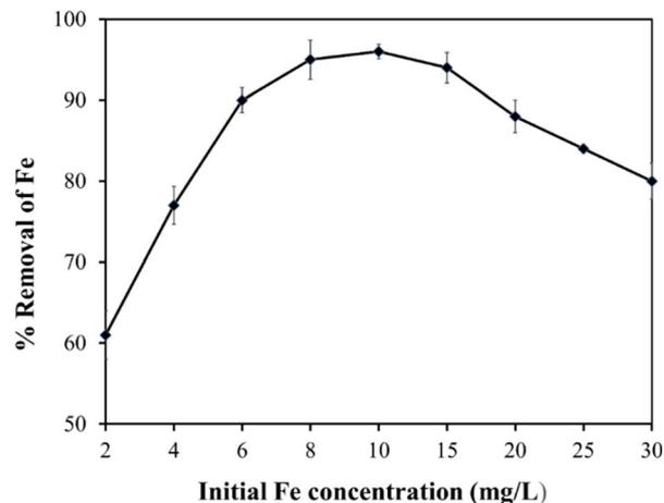
Fig. 10 Effect of the initial metal concentration on Fe removal efficiency.
