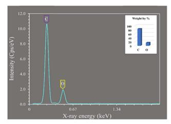
Fig. 2 The EDX micrograph illustrates the existence of carbon and oxygen in the biochar derived from baobab seeds after pyrolysis at  $700^{\circ}$ C
