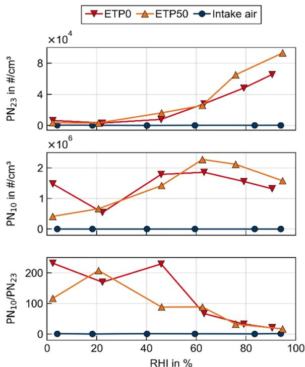
Fig. 4  $PN_{23}$ ,  $PN_{10}$ , and  $PN_{10}/PN_{23}$  ratio in motored operation with additional PN in intake air for variations of the relative humidity in the intake and the exhaust throttle position.
