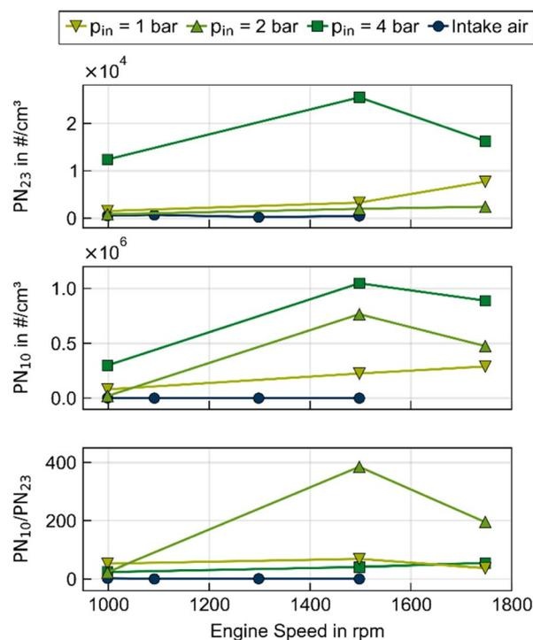
Fig. 3  $PN_{23}$ ,  $PN_{10}$ , and  $PN_{10}/PN_{23}$  ratio in motored operation with additional PN in intake air for variations of the engine speed and the engine's supercharging level, defined as  $p_{in}$ .
