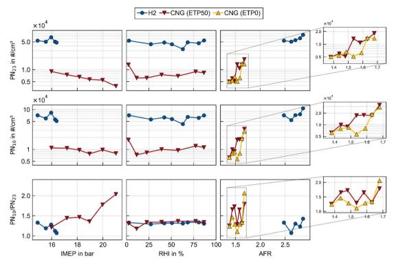
Fig. 7  $PN_{23}$ ,  $PN_{10}$ , and  $PN_{10}/PN_{23}$  ratio in hydrogen and natural gas operations for variations of AFR, IMEP, and the relative humidity in the intake, additionally varying the exhaust throttle position in natural gas operation.
