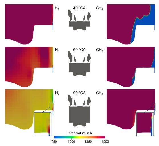
Fig. 9 3D CFD simulations of hydrogen and methane combustion at an AFR = 2.5 for hydrogen operation and AFR = 1.5 for methane operation at 1500 rpm, comparing flame propagation and flame quenching distance for 40 °CA, 60 °CA and 90 °CA after TDC.
