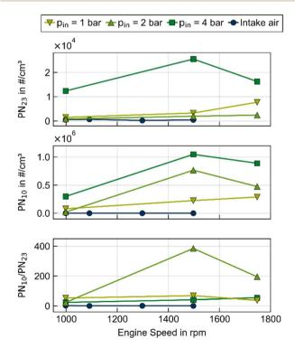
Fig. 3  $PN_{23}$ ,  $PN_{10}$ , and  $PN_{10}/PN_{23}$  ratio in motored operation with additional PN in intake air for variations of the engine speed and the engine's supercharging level, defined as  $p_{\rm in}$ .
