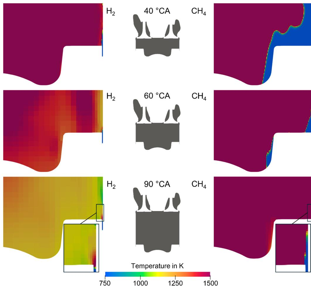
Fig. 9 3D CFD simulations of hydrogen and methane combustion at an AFR = 2.5 for hydrogen operation and an AFR = 1.5 for methane operation at 1500 rpm, comparing flame propagation and flame quenching distance for 40 °CA, 60 °CA and 90 °CA after TDC.
