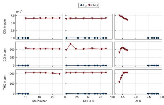
$\textbf{Fig. 8} \quad \textbf{Absolute CO}_2, \textbf{CO}, \textbf{and THC emissions in hydrogen and natural gas operations for variations of AFR, IMEP, and the relative humidity in the} \\$ intake.
