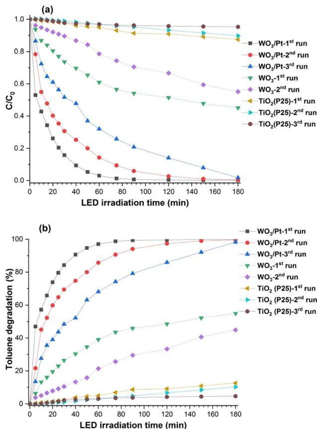
Fig. 7 (a) Plots of  $C/C_0$  vs. visible light (LED) irradiation time inside the photoreactor with  $WO_3/Pt$ , pure  $WO_3$ , and  $TiO_2$ ;  $C_0$  represents the concentration of toluene (in ppm) before switching ON the LED light, and  $C$  is the toluene concentration with respect to the LED light exposure duration (in min), and (b) plots of toluene degradation (%) as a function of LED light exposure time.
