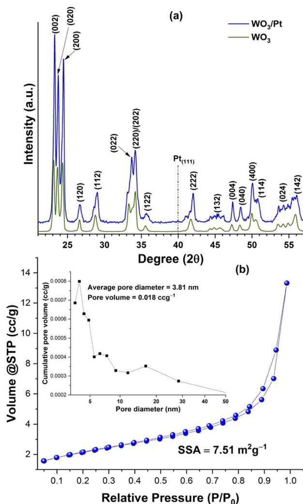
Fig. 2 (a) XRD pattern of the  $\text{WO}_3/\text{Pt}$  nanocomposite and pure  $\text{WO}_3$  powder; the corresponding  $hkl$  planes of the respective diffraction peaks are indexed in the graph. (b)  $\text{N}_2$  adsorption-desorption isotherm and pore-size distribution (inset) of the  $\text{WO}_3/\text{Pt}$  nanocomposite.
