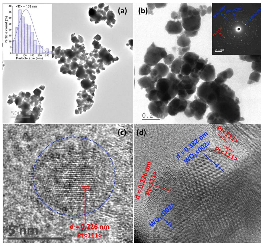
Fig. 3 (a and b) Bright-field TEM images of the  $\text{WO}_3/\text{Pt}$  nanoparticles, along with a histogram of the particle-size distribution (inset of (a)) and the corresponding SAED pattern (inset of (b)). (c and d) HRTEM images at different magnifications: (a and b) low magnification images showing the distribution of the  $\text{WO}_3/\text{Pt}$  nanoparticles.
