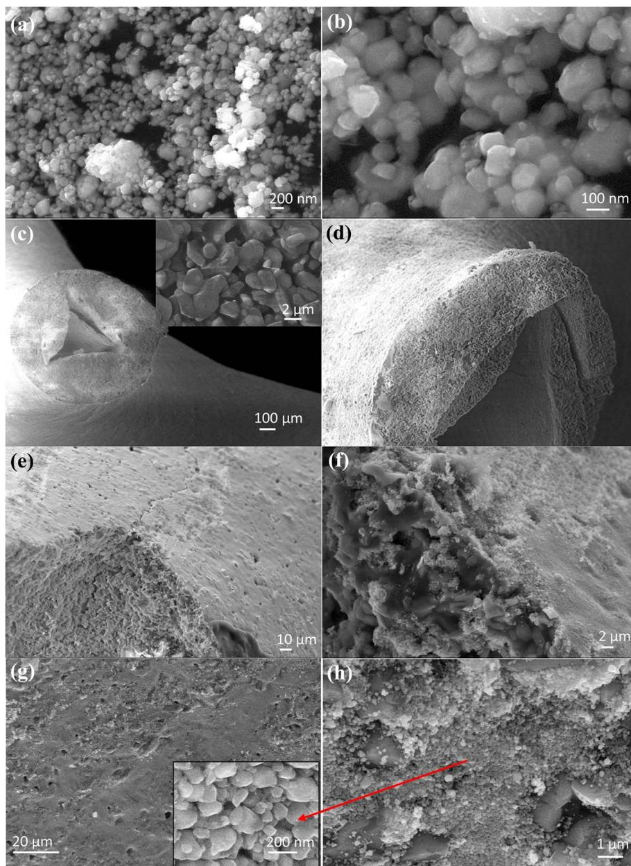
Fig. 6 FESEM images of (a) and (b)  $\text{WO}_3/\text{Pt}$  particles; (c) and (d) bare ceramic filter, and (e–h)  $\text{WO}_3/\text{Pt}$ -coated ceramic filter at different magnifications.
