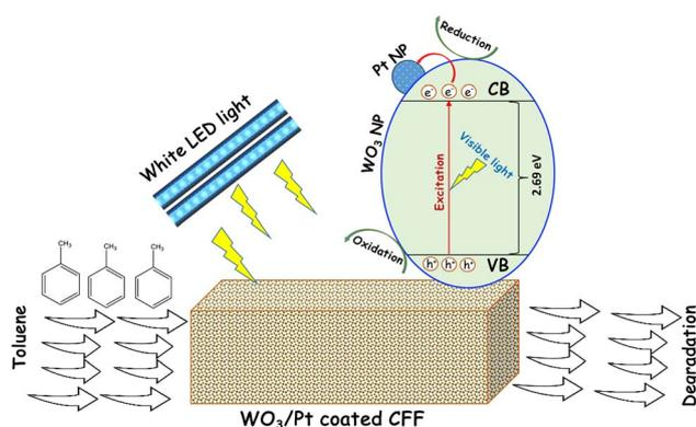
Fig. 9 Schematic of the proposed toluene photodegradation mechanism by the  $\text{WO}_3/\text{Pt}$ -coated CFF under visible light irradiation.
