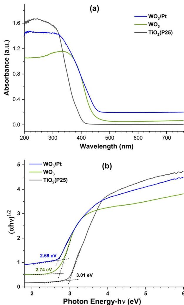
Fig. 4 (a) UV-visible diffuse reflectance spectra in the absorbance scale of the WO<sub>3</sub>/Pt nanocomposite powder, pure WO<sub>3</sub> powder, and commercial TiO<sub>2</sub> (P25) powder. (b) Plots of  $(\alpha h\nu)^{1/2}$  against the photon energy  $h\nu$  (eV) for the respective samples.
