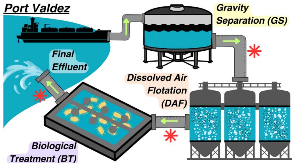
Fig. 1 Overview of the ballast water treatment facility at the Valdez Marine Terminal. Green arrows represent flow direction, and red asterisks represent a sampling point.
