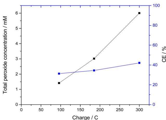
Fig. 2 Peroxide formation during chronocoulometry at 2.385 V vs. Ag/AgCl using a  $\text{BiVO}_4$  anode. Total charge of 300 C passed during the experiment. Conditions:  $3.75 \text{ cm}^2$   $\text{BiVO}_4$  working electrode (anode),  $4.9 \text{ cm}^2$  gas diffusion electrode (cathode), divided cell (cation exchange membrane), 110 mL 0.5 M  $\text{KHCO}_3$  and 3.5 M  $\text{K}_2\text{CO}_3$  in each chamber.
