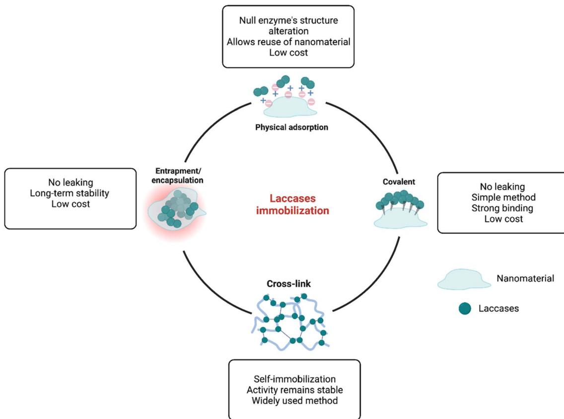
Fig. 4 Routes for laccase immobilization into nanomaterials.
