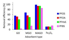
Fig. 8 Removal efficiency of different adsorbents for PFAS compounds. Conditions: 40 mL of 500  $\mu$ g L<sup>-1</sup> PFAS, pH 6.5, 20 mg adsorbent, and 60 min extraction time.
