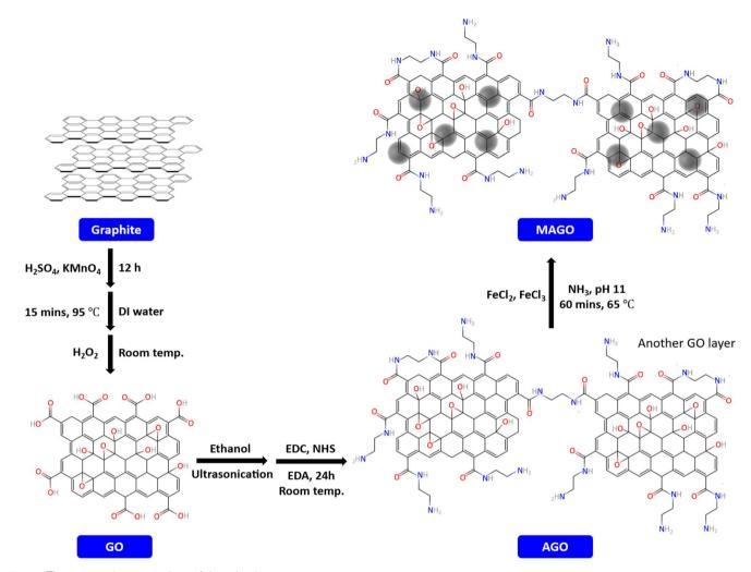
Fig. 1 The preparation procedure of the adsorbent.
