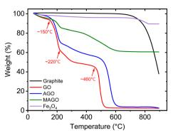
Fig. 7 TGA curves of pristine graphite, GO, AGO, MAGO, and Fe<sub>3</sub>O<sub>4</sub>.
