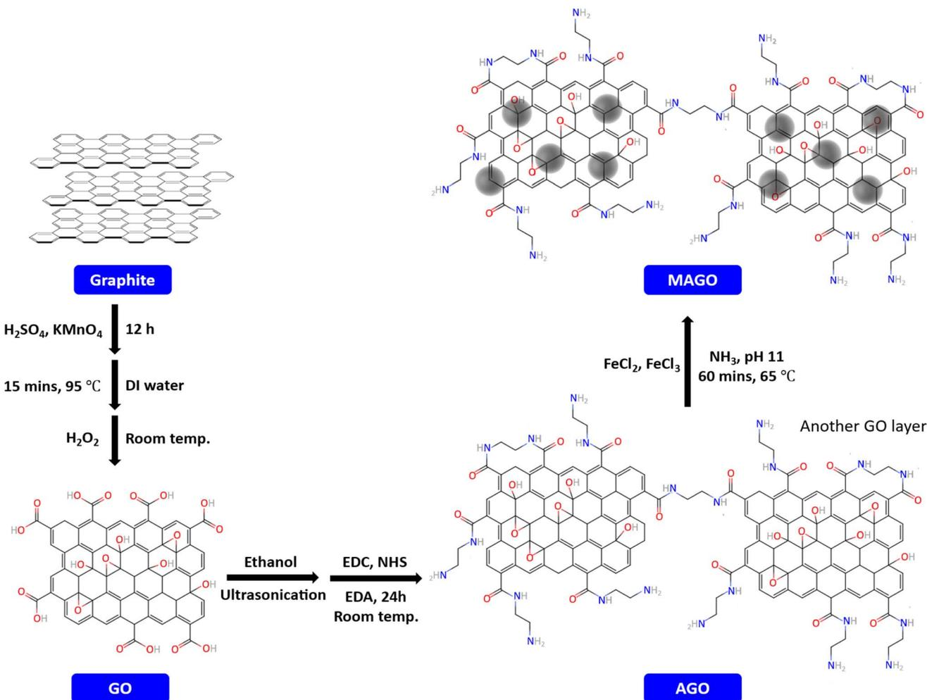
Fig. 1 The preparation procedure of the adsorbent.
