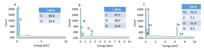
Fig. 5 The EDS spectra of (a) GO, (b) AGO, and (c) MAGO
