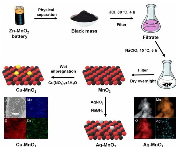
Fig. 1 Synthesis methodology for preparing Cu–MnO<sub>2</sub> (ref. 27) and Ag–MnO<sub>2</sub> catalysts.<sup>35</sup> EDX mapping of Cu–MnO<sub>2</sub> reproduced from ref. 27 with permission from Elsevier, copyright 2024. EDX mapping of Ag–MnO<sub>2</sub> reproduced with minor modification from ref. 35 with permission from The Royal Society of Chemistry, copyright 2024.
