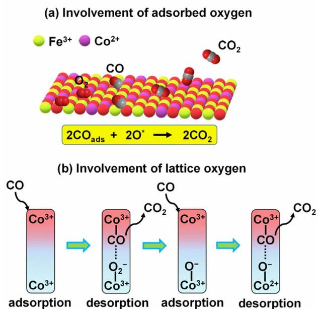
Fig. 4 The role of  $\text{CoFe}_2\text{O}_4$ -LIBs catalyst in CO oxidation involves the interaction of CO with (a) adsorbed oxygen species over  $\text{CoFe}_2\text{O}_4$  and (b) lattice oxygen over  $\text{Co}_3\text{O}_4$ .<sup>41</sup>
