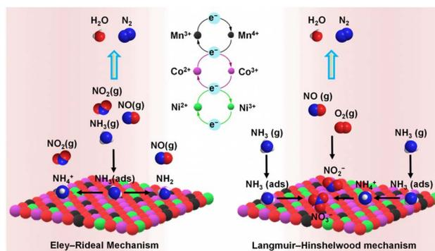
Fig. 5 Proposed  $\text{NH}_3$ -SCR mechanism for NO conversion to  $\text{N}_2$  over waste LIBs-derived  $\text{NiCoMnO}_x$  catalyst.<sup>37</sup>
