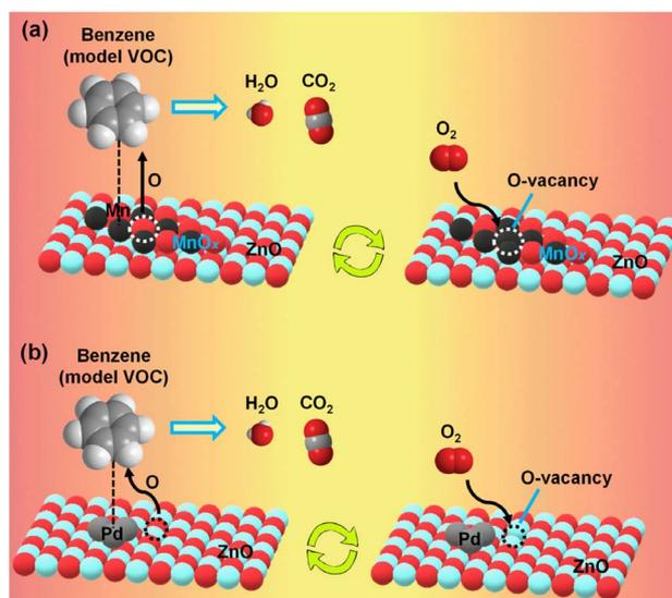
Fig. 3 Proposed reaction mechanism for complete oxidation of BTX molecules over (a) MnO<sub>x</sub>–ZnO<sup>52</sup> (b) Pd–ZnO.<sup>33</sup>
