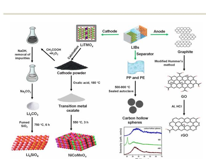
Fig. 2 A schematic illustration of synthesis methodologies adopted for processing LIB's components into functional materials.<sup>37,39,40</sup> The PXRD pattern of synthesised carbon materials reproduced with minor modification from ref. 40 with permission from The Royal Society of Chemistry, copyright 2024.
