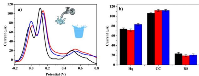
Fig. 8 (a) Square wave voltammograms using ZrO<sub>2</sub>10Sc/SPCE in a solution containing 300  $\mu\text{M}$  HQ, CC and RS in 0.01 M PBS at pH = 7.4 (black line), in tap water (red line) and in mineral water (blue line). (b) Peak anodic currents ( $I_{pa}$ ) are shown in the diagram (SD  $\leq$  2.6 for 3 times).
