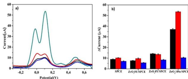
Fig. 4 (a) Square-wave voltammograms using the bare SPCE (black line), ZrO<sub>2</sub>OY/SPCE (red line), ZrO<sub>2</sub>8Y/SPCE (blue line) and ZrO<sub>2</sub>10Sc/SPCE (green line) in a solution containing 100 μM HQ and CC in 0.01 M PBS at pH = 7.4. (b) Comparison of the variation in the intensity of anodic current peaks (*I*<sub>pa</sub>) obtained for the DHBs (HQ = black, CC = red, RS = blue) on the different sensors (SD ≤ 0.75 for 3 times).
