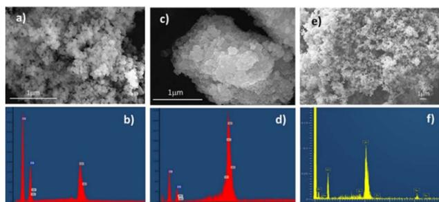
Fig. 1 SEM image and EDX of (a) and (b)  $\text{ZrO}_2\text{OY}$  sample; (c) and (d)  $\text{ZrO}_2\text{8Y}$  sample; (e) and (f)  $\text{ZrO}_2\text{10Sc}$  sample.
