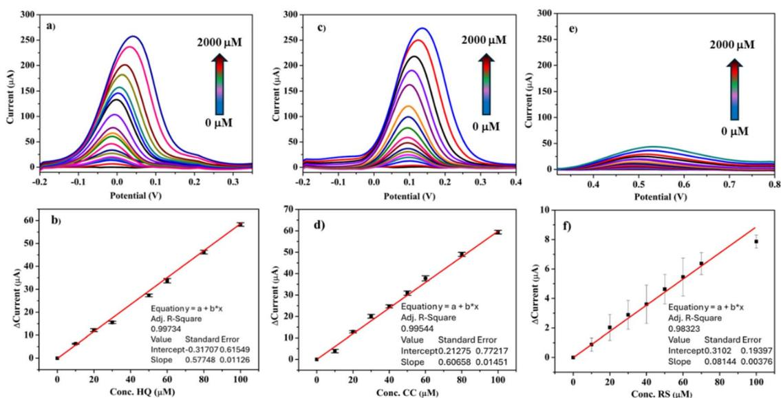
Fig. 5 SWV of (a) HQ, (c) CC and (e) RS standard solutions with increasing concentrations from 0 to 2000 μM of analytes recorded in a 0.01 M PBS of pH = 7.4 using ZrO<sub>2</sub>10Sc/SPCE. Calibration graphs for peak currents (baseline corrected) as a function of analyte concentrations of (b) HQ (SD ≤ 0.95 for 3 times), (d) CC (SD ≤ 1.2 for 3 times), and (f) RS (SD ≤ 1.29 for 3 times).
