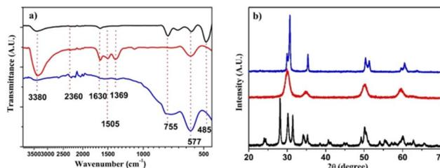
Fig. 2 (a) FT-IR analysis of the investigated samples,  $\text{ZrO}_2\text{OY}$  (black line),  $\text{ZrO}_2\text{8Y}$  (red line), and  $\text{ZrO}_2\text{10Sc}$  (blue line). (b) XRD analysis of the investigated samples  $\text{ZrO}_2\text{OY}$  (black line),  $\text{ZrO}_2\text{8Y}$  (red line), and  $\text{ZrO}_2\text{10Sc}$  (blue line).
