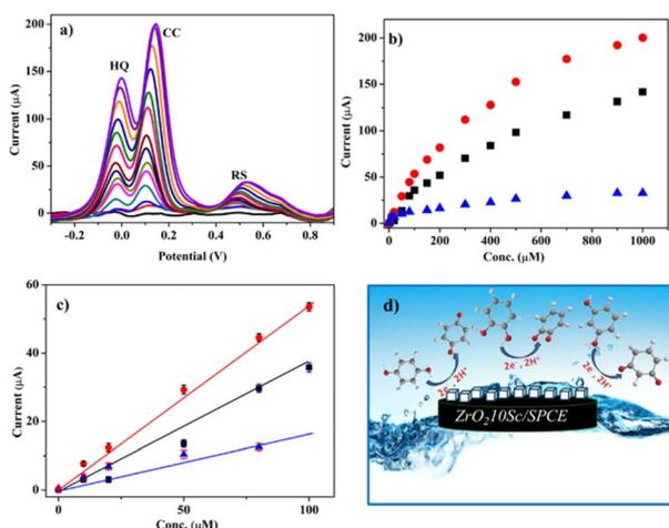
Fig. 7 (a) Simultaneous measurement of HQ (black curve), CC (red curve) and RS (blue curve) in the range of 0 to 1000  $\mu M$  DHB isomers in solution; (b) calibration graphs for peak currents (baseline corrected) as a function of analyte concentrations ( $SD \leq 1.18$  for 3 times); (c) linear range (0–100  $\mu M$ ) of the calibration curves of HQ (black curve), CC (red curve) and RS (blue curve); (d) schematic diagram of the DHB isomer mechanism at the  $ZrO_2$ 10Sc/SPCE interface.
