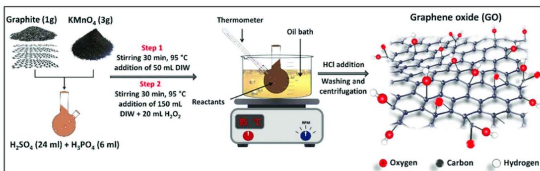
Fig. 1 GO synthesis by a modified Hummer's method.<sup>57</sup>
