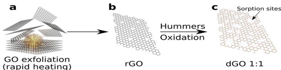
Fig. 7 Scheme for the preparation of defective GO: (a) explosive thermal-exfoliation of GO, (b) Hummer's oxidation of defective rGO and (c) dGO with sorption sites.<sup>219</sup>
