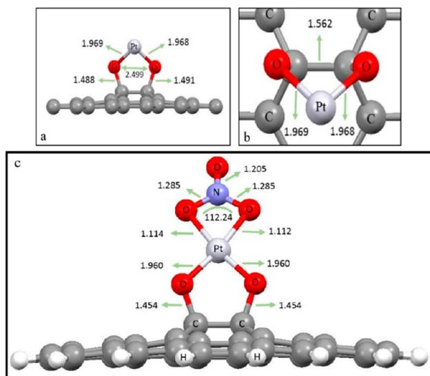
Fig. 8 (a and b) Side view and top view of the optimized position of Pt-nanoparticles on the surface of GO, and (c) optimized nitrate-interaction with the GO/Pt surface and bond lengths (Å).<sup>199</sup>
