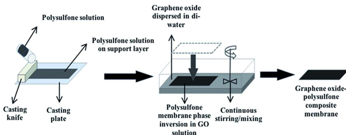
Fig. 2 Phase inversion method for generation of a PSF membrane.<sup>68</sup>
