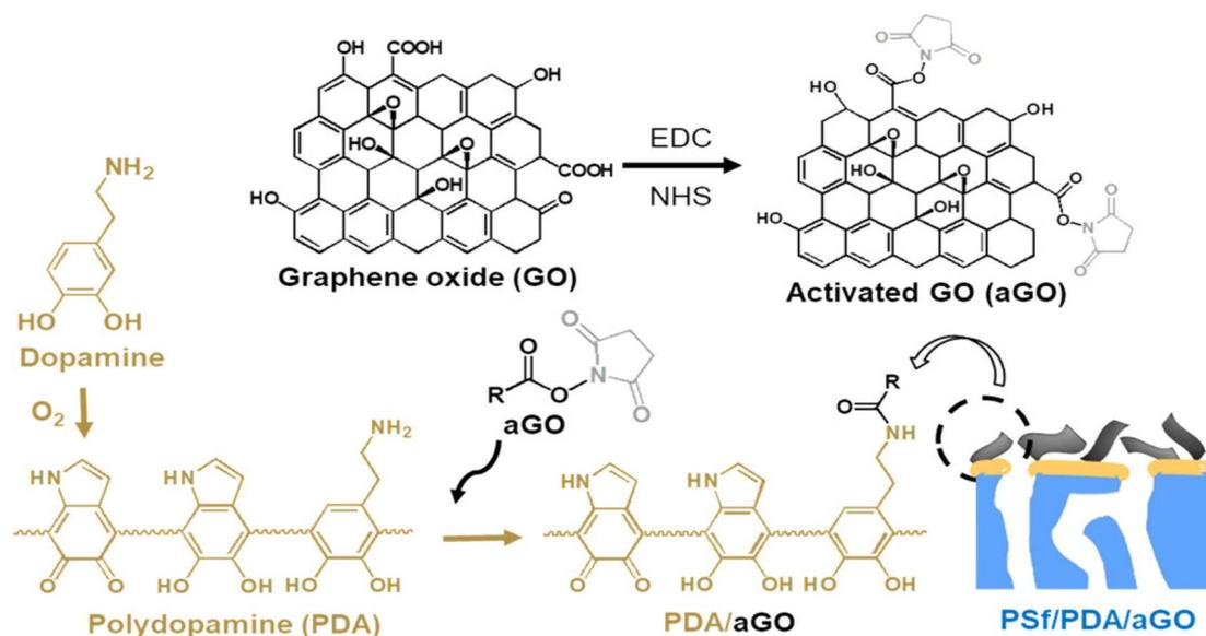
Fig. 6 Modification of a graphene oxide based polydopamine coated polysulfone (GO-PDA-PSF) membrane using 1-ethyl-3-(3-dimethylaminopropyl)carbodiimide (EDC) and *N*-hydroxysuccinimide (NHS).<sup>131</sup>
