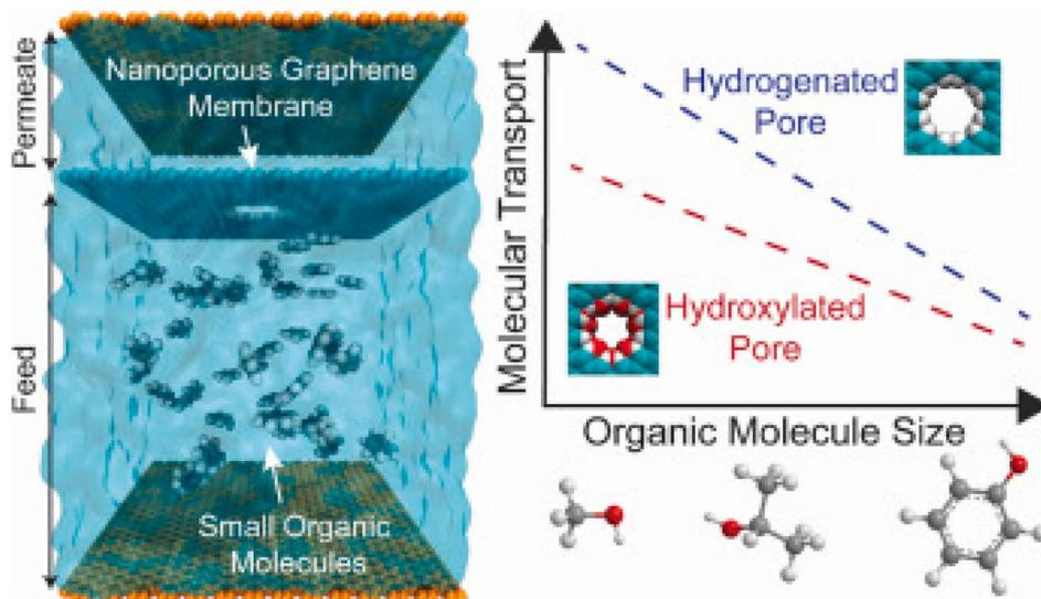
Fig. 9 Illustration of the performance of the NPG membrane for the removal of organic molecules.<sup>229</sup>
