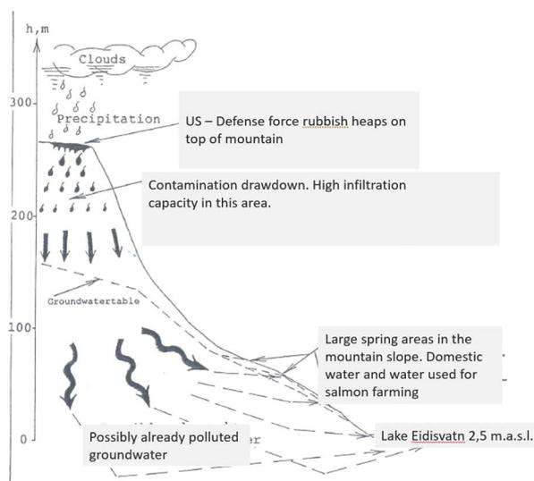
Fig. 2 Transport model of pollution spread at Heiðarfjall.<sup>42</sup>
