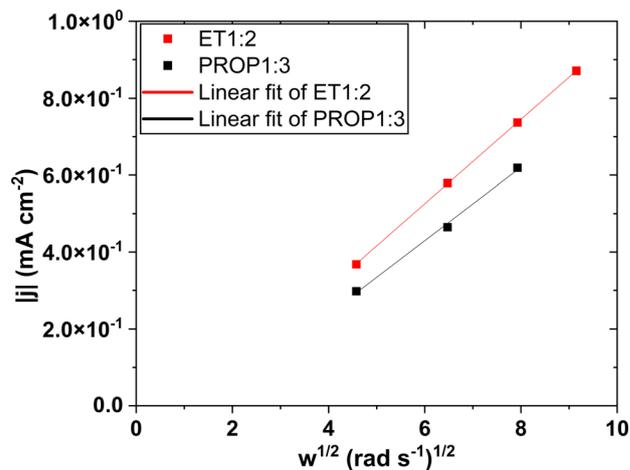
Fig. 7 Variations of the current density of the rotating disk electrode under mass transfer control with the square root of the angular velocity  $\omega$ . The solid line corresponds to Levich's law (6).
