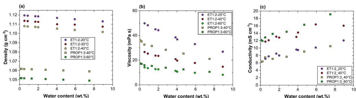
Fig. 1 Experimental transport properties of the two DES depending on temperature and their water content; (a) density of ET1:2 and PROP1:3; (b) viscosity of ET1:2 and PROP1:3; (c) ionic conductivity of ET1:2 and PROP1:3.
