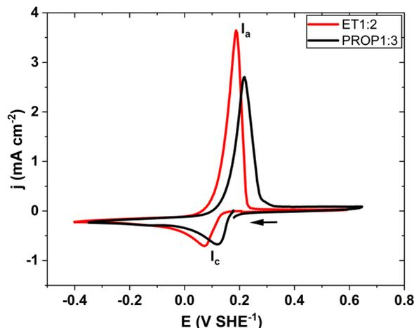
Fig. 5 Cyclic voltammetry at  $20 \text{ mV s}^{-1}$  of the electroleachate of silver (25 mM) in PROP1:3 (in black) and in ET1:2 (in red) with 3.5 wt% of water content.
