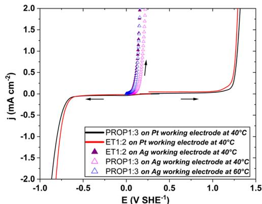
Fig. 3 Electrochemical windows of the two DES revealed by linear sweep voltammograms on a Pt surface at 40 °C,  $10 \text{ mV s}^{-1}$  in the range  $-0.75/1.3 \text{ V SHE}^{-1}$  (solid lines). Besides, linear sweep voltammograms on an Ag surface at  $10 \text{ mV s}^{-1}$  in the two DES are also given: ET1:2 at 40 °C ( $\blacktriangle$ ) and in PROP1:3 at 40 °C ( $\blacktriangle$ ) and at 60 °C ( $\blacktriangle$ ).
