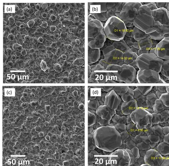
Fig. 9 SEM view of Ag deposits formed at  $-0.25 \text{ mA cm}^{-2}$  at  $60 \text{ }^\circ\text{C}$  from Ag(I) solutions of ET1:2 (photo (a) and its zoom (b)), and PROP1:3 (photo (c) and its zoom (d)); Ag(I) concentration equal to  $57 \pm 2 \text{ mmol L}^{-1}$ ; charge passed near  $22 \text{ A s cm}^{-2}$ .
