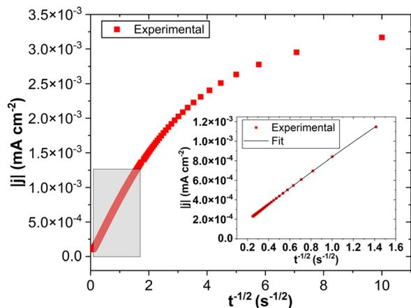
Fig. 6 Chronoamperometric test under mass control for Ag(I) at 25 mM in ET1:2 at 40 °C: transient of the current density recorded. Inset, variation of the current density with time to the power  $\frac{1}{2}$  after Cottrell's law. The grey-colored area indicates the time considered in  $D$  determination.
