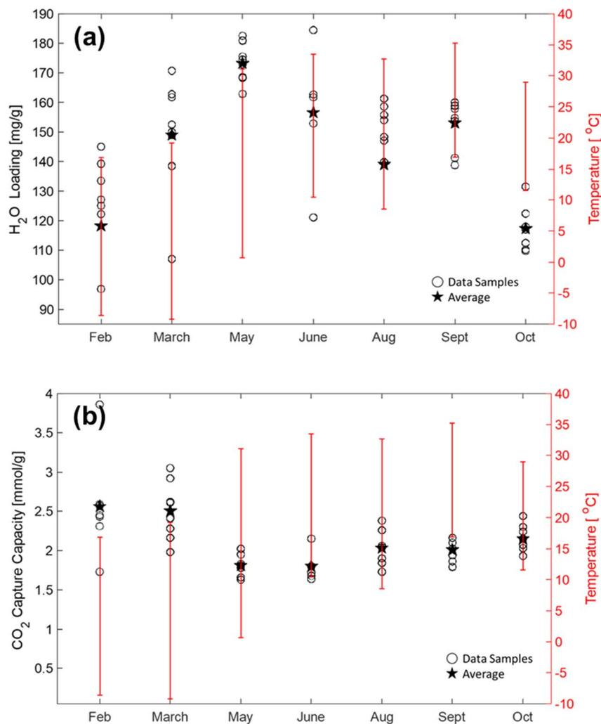
Fig. 5 Results of monthly RTU H<sub>2</sub>O (a) and CO<sub>2</sub> loading (b) from February to October 2022.
