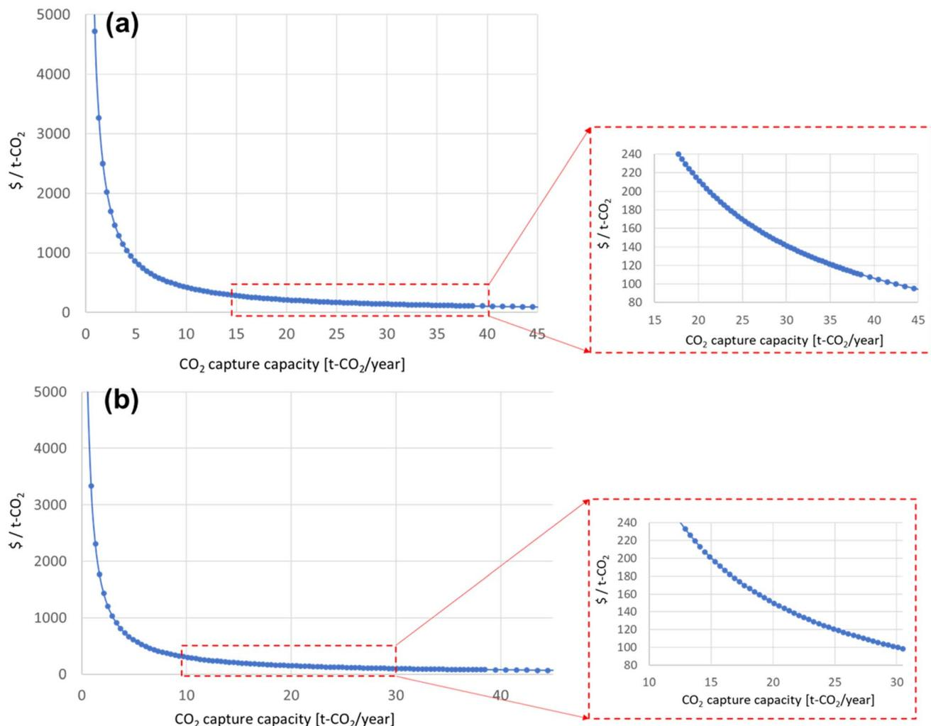
Fig. 8 Levelized cost of CO<sub>2</sub> capture based on assumed CO<sub>2</sub> capture capacity: (a) 5 year analysis and (b) 10 year analysis.
