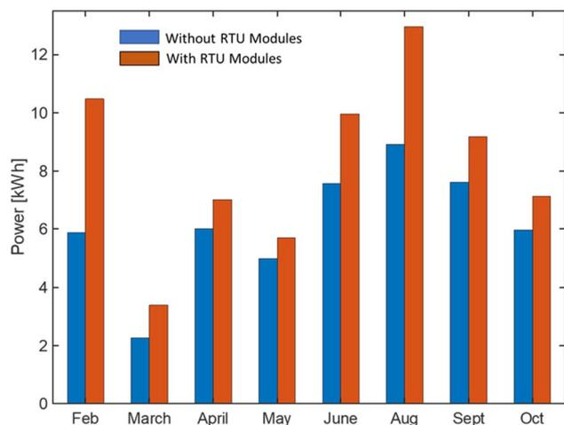
Fig. 6 Comparison of additional hourly power consumption with and without RTU modules for February to October 2022.
