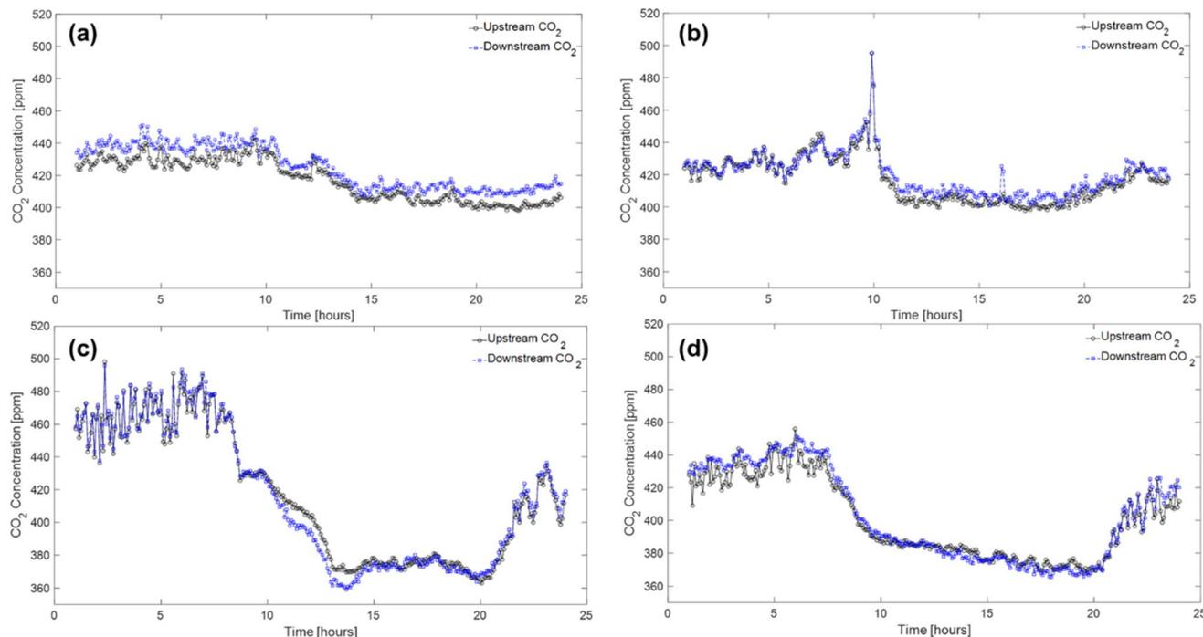
Fig. 4 Profiles of CO<sub>2</sub> upstream and downstream concentrations with (a and c) and without (b and d) the RTU modules during February (a and b) and June (c and d) 2022.
