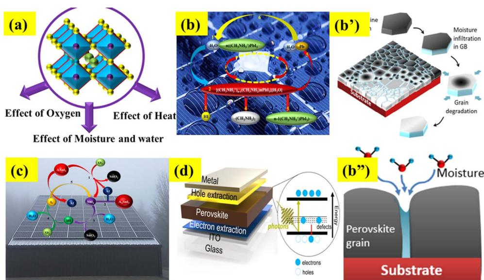
Fig. 4 (a) External factor effect on the stability of PSCs, (b–b’’) effect of water and moisture. Reproduced with permission.<sup>114</sup> Copyright 2015, American Chemical Society. (c) Influence of oxygen and (d) analysis of the heat effect.
