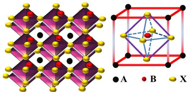
Fig. 1 Schematic diagram of the crystal structure of PSCs.<sup>32</sup>
