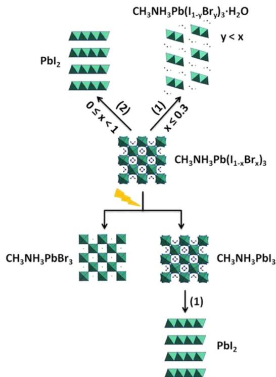
Fig. 5 Diagram of degradation of MAPb(I<sub>1-x</sub>Br<sub>x</sub>)<sub>3</sub> exposed to humidity.<sup>151</sup>
