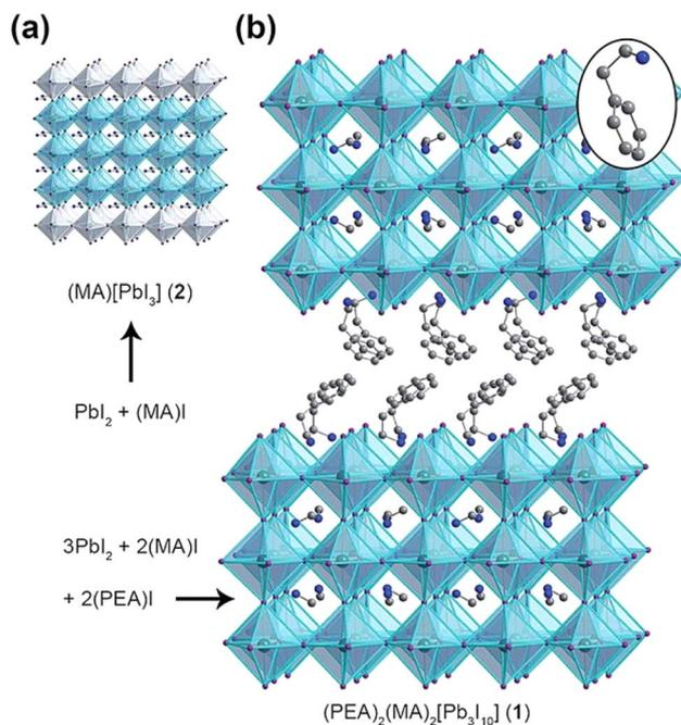
Fig. 6 Crystal structures of (a) 3D perovskite MAPbI<sub>3</sub> and (b) 2D perovskite PEA<sub>2</sub>MA<sub>2</sub>Pb<sub>3</sub>I<sub>10</sub>.<sup>153</sup>
