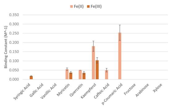
Fig. 7 Calculated binding constant values for the model compounds chosen (with error bars showing standard deviation for triplicate experiments).
