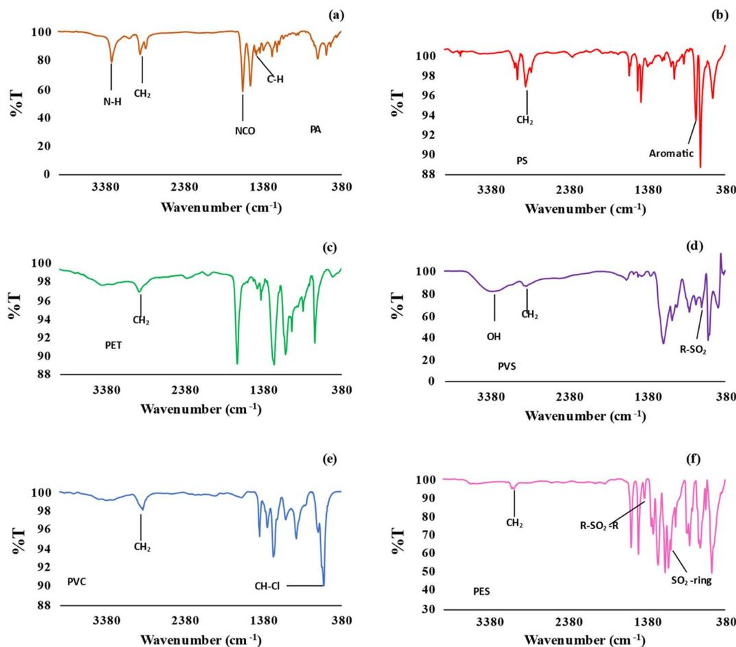
Fig. 3 IR absorption spectrum for PA (a), PS (b), PET (c), PVS (d), PVC (e), and PES (f).
