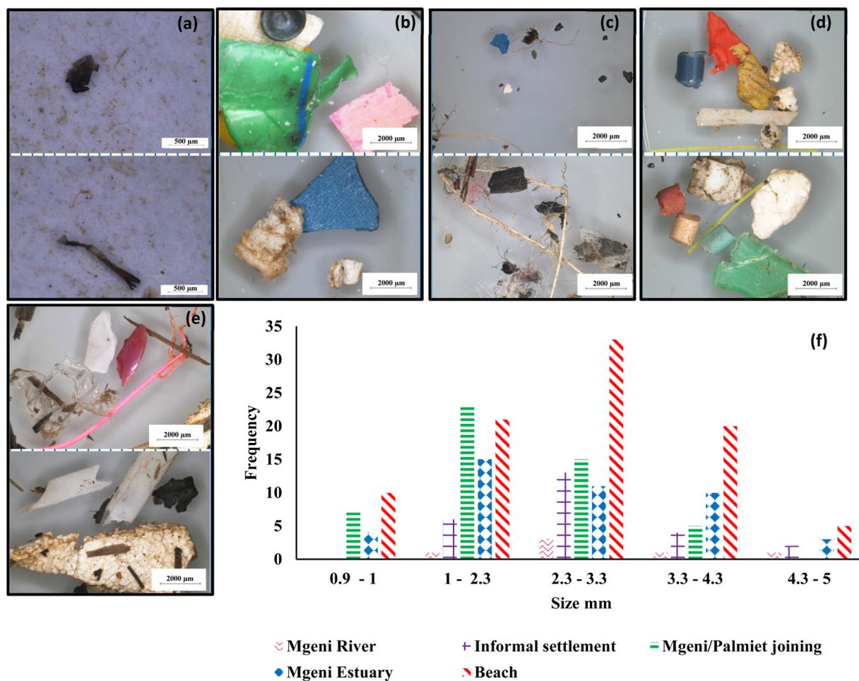
Fig. 6 Micrographs for environmental samples from the Mgeni River before joining (a), informal settlement (Palmiet River) (b), joining Palmiet/Mgeni River (c), uMgeni Estuary (d) and ocean (e) with the histogram for microplastic size (f).
