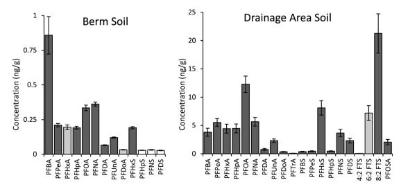
Fig. 1 Fall concentrations of PFAS in field soils from berm and drainage area. Error bars represent standard error (berm soil  $7 \le n \le 32$ , drainage area soil  $6 \le n \le 8$ , non-detects not included in calculations). Bar color indicates detection frequency: dark gray 100%, medium gray 75–99%, and white below 74%. Data for PFOS is not shown (7.5 ng  $g^{-1}$  in berm soil and 107 ng  $g^{-1}$  in drainage area soil).
