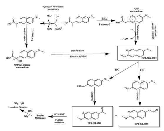
Fig. 13 Overall degradation mechanism of NAP in the UVA/MIL-88-A/PS system
