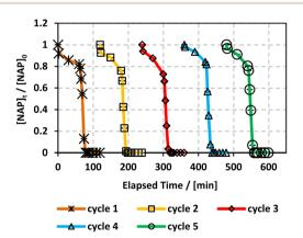
Fig. 6 Recyclability experiments of MIL-88-A in solar/MIL-88-A/PS/NAP system. [NAP] $_0=50~\text{mg L}^{-1}$ , [PS] $_0=2~\text{mM}$ , [MIL-88-A] $_0=25~\text{mg L}^{-1}$ . Error bars are calculated as  $\frac{ts}{\sqrt{n}}$  where absent bars fall within the symbols.
