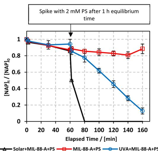
Fig. 3 Elimination of NAP in a combined MIL-88-A/PS system and the presence of solar or UVA light. Experimental conditions:  $[NAP]_0 = 50 \text{ mg L}^{-1}$ ,  $[PS]_0 = 2 \text{ mM}$ ,  $[MIL-88-A]_0 = 25 \text{ mg L}^{-1}$ . Error bars are calculated as  $\frac{ts}{\sqrt{n}}$ , where absent bars fall within the symbols.
