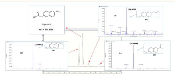
Fig. 12 HPLC chromatogram at T = 25 °C showing NAP and its by-products at reaction time t = 100 min. Analysis was done on Thermo Ultimate 3000 UHPLC with HR mass spectrum fragmentation pattern of (a) BP1, (b) BP2 and (c) BP3.
