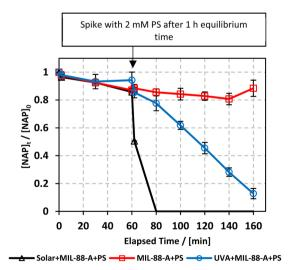
Fig. 3 Elimination of NAP in a combined MIL-88-A/PS system and the presence of solar or UVA light. Experimental conditions: [NAP] $_0=50~{\rm mg~L}^{-1}$ , [PS] $_0=2~{\rm mM}$ , [MIL-88-A] $_0=25~{\rm mg~L}^{-1}$ . Error bars are calculated as  $\frac{ts}{\sqrt{n}}$ , where absent bars fall within the symbols.
