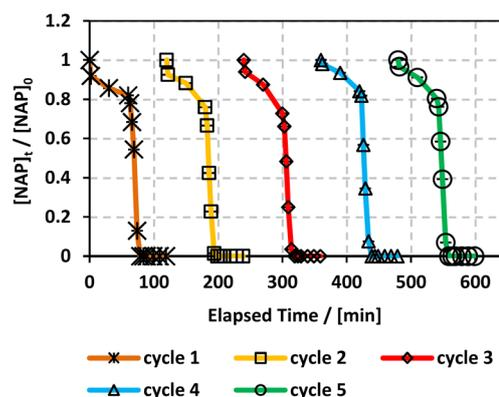
Fig. 6 Recyclability experiments of MIL-88-A in solar/MIL-88-A/PS/NAP system.  $[\text{NAP}]_0 = 50 \text{ mg L}^{-1}$ ,  $[\text{PS}]_0 = 2 \text{ mM}$ ,  $[\text{MIL-88-A}]_0 = 25 \text{ mg L}^{-1}$ . Error bars are calculated as  $\frac{ts}{\sqrt{n}}$ , where absent bars fall within the symbols.
