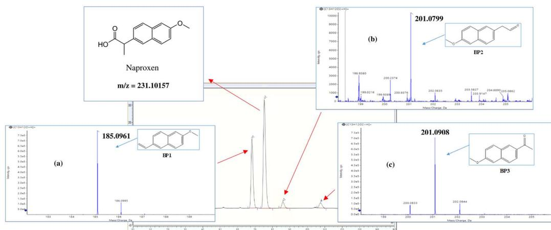
Fig. 12 HPLC chromatogram at  $T = 25\text{ }^{\circ}\text{C}$  showing NAP and its by-products at reaction time  $t = 100\text{ min}$ . Analysis was done on Thermo Ultimate 3000 UHPLC with HR mass spectrum fragmentation pattern of (a) BP1, (b) BP2 and (c) BP3.
