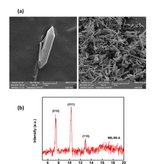
Fig. 2 Characterization of the synthesized MIL-88-A: (a) SEM of MIL-88-A crystals at different magnifications (b) XRD diffraction pattern.
